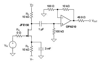
Figure 7-1. AC Measurement Reference Schematic
