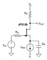
Figure 9-4. Common-Source Amplifier With Current-Source Biasing
