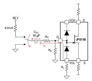
Figure 9-1. JFE150 Clamping Diode Example
