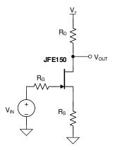
Figure 9-2. Common-Source Amplifier
