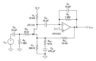
Figure 9-6. Low-Noise, High-Input-Impedance Composite Amplifier
