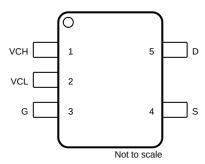
Figure 5-1. DBV, 5-Pin SOT-23 and DCK, 5-Pin SC70 Packages (Top View)
