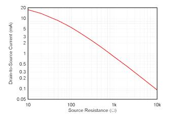
Figure 9-3. Drain-to-Source Current vs  $R_S$ ,  $V_{DS} = 5 V$
