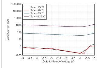
Figure 6-5. Gate Current vs Drain-to-Source Voltage
