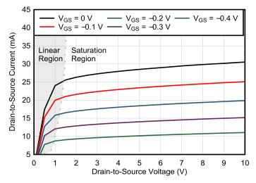
Figure 8-1. V<sub>DS</sub> vs I<sub>DS</sub>
