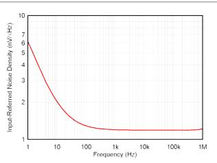
Figure 9-8. Input-Referred Noise Density
