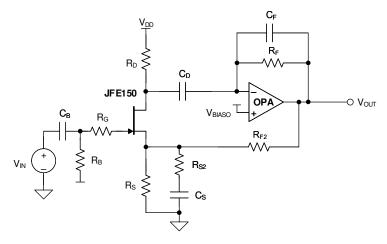
Figure 9-5. Low Noise, High Input Impedance Composite Amplifier
