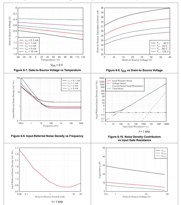
Figure 6-11. Input-Referred Noise Spectral Density
