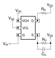
Figure 9-9. JFE150 Layout Example, Common Source Configuration
