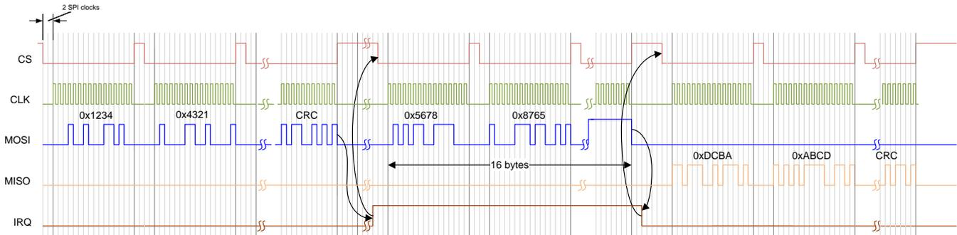
**Figure 5-10. SPI Communication**
