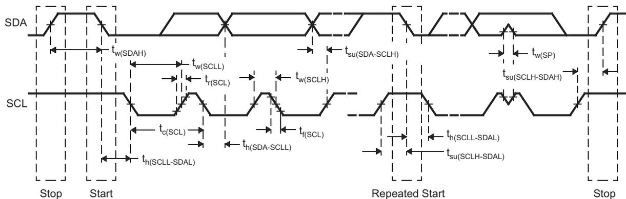
**Figure 5-13. I2C Timing Diagram****NOTE**
