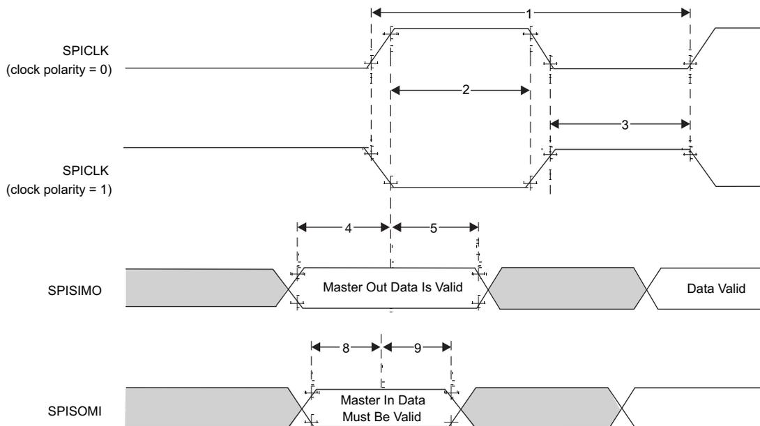
**Figure 5-6. SPI Master Mode External Timing (CLOCK PHASE = 1)**
