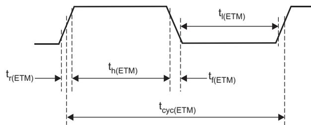
**Figure 5-16. ETMTRACECLKOUT Timing**
