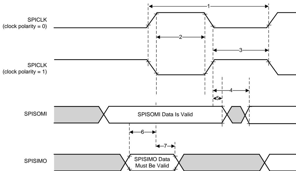
Figure 5-9. SPI Slave Mode External Timing (CLOCK PHASE = 1)
