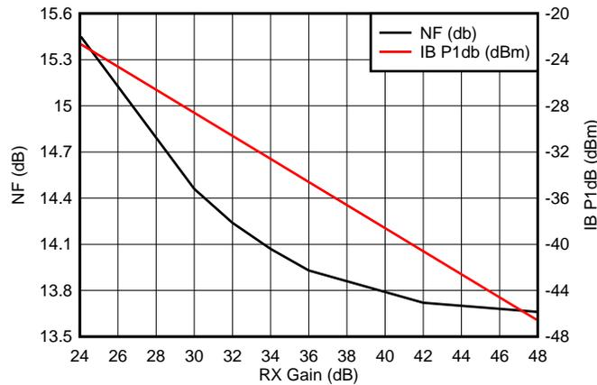
Figure 5-1. Noise Figure, In-band P1dB vs Receiver Gain
