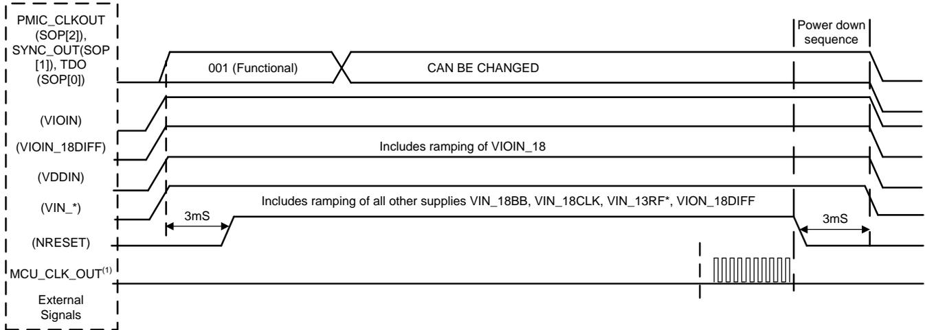
(1) MCU\_CLK\_OUT in autonomous mode, where IWR1642 application is booted from the serial flash, MCU\_CLK\_OUT is not enabled by default by the device bootloader.
