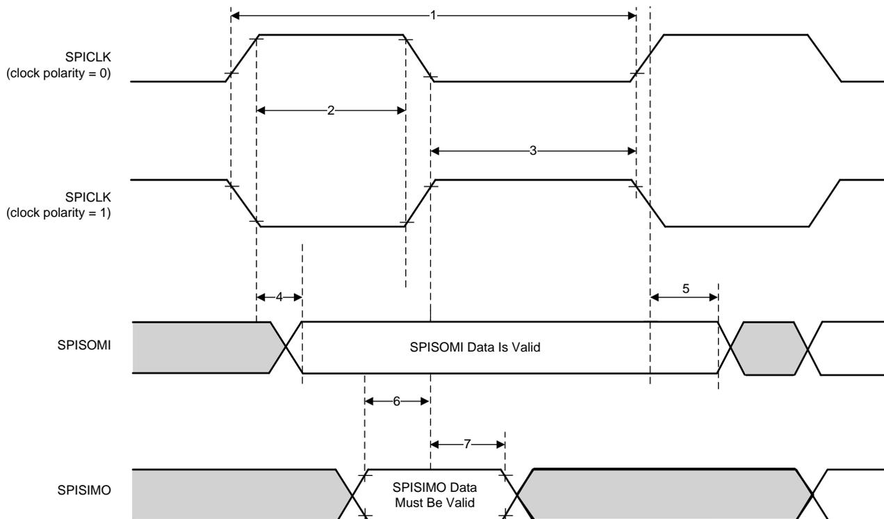
Figure 5-8. SPI Slave Mode External Timing (CLOCK PHASE = 0)
