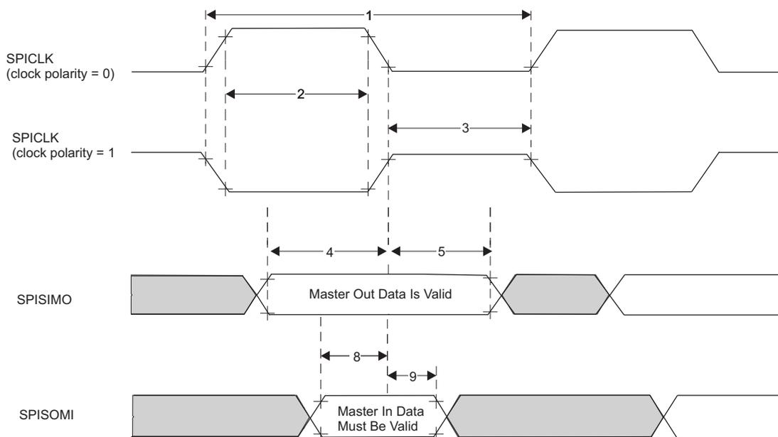
**Figure 5-4. SPI Master Mode External Timing (CLOCK PHASE = 0)**
