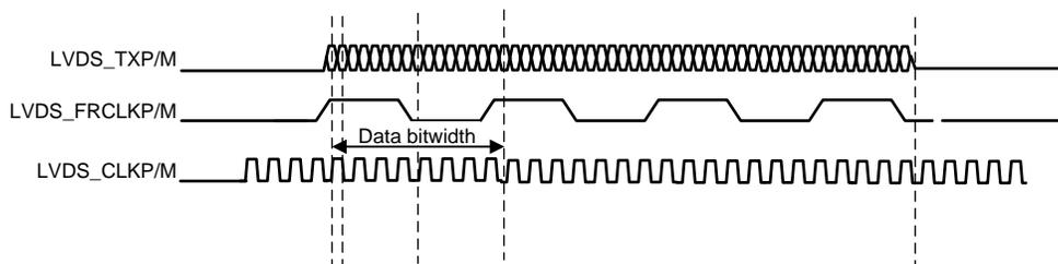
Figure 5-11. LVDS Interface Lane Configuration And Relative Timings
