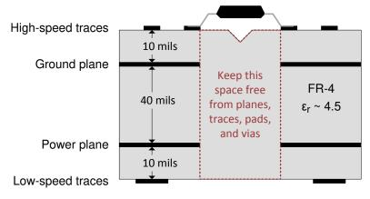
Figure 8-4. Layout Example Schematic
