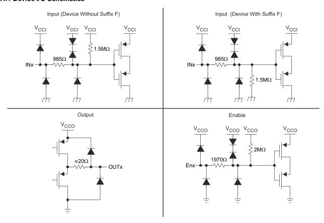
Figure 7-3. Device I/O Schematics
