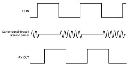
Figure 7-2. On-Off Keying (OOK) Based Modulation Scheme
