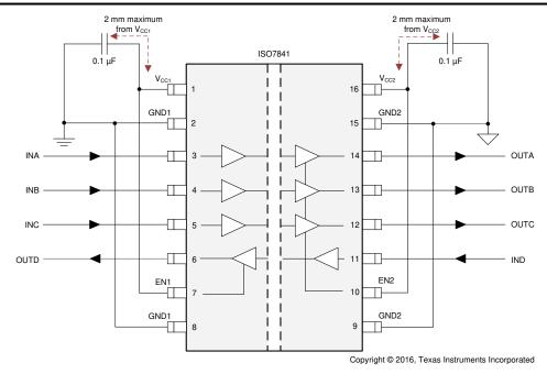
Figure 8-2. Typical ISO7841 Circuit Hook-Up
