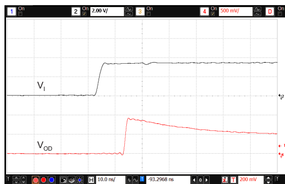
Figure 15. Distortion Correction Scheme Calibration Time ( t_{CALIB} )
