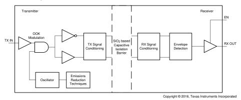
Figure 7-1. Conceptual Block Diagram of a Digital Capacitive Isolator
