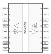
Figure 4-1. DW Package 16-Pin (SOIC) Top View
