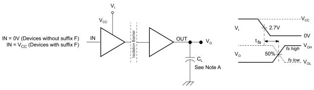
A.  $C_L = 15 \text{ pF}$  and includes instrumentation and fixture capacitance within  $\pm 20\%$ .
