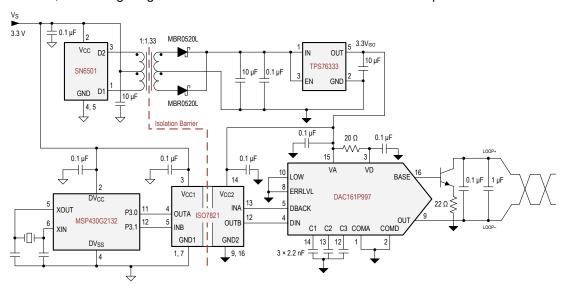
Figure 8-1. Isolated 4-20 mA Current Loop
