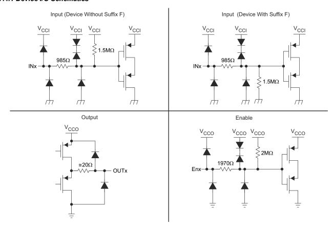
Figure 7-3. Device I/O Schematics
