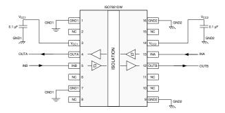
Figure 8-2. Typical ISO7821 Circuit Hook-up
