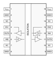
Figure 4-2. DWW Package 16-Pin (SOIC) Top View
