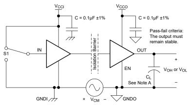
A.  $C_L = 15 \text{ pF}$  and includes instrumentation and fixture capacitance within  $\pm 20\%$ .
