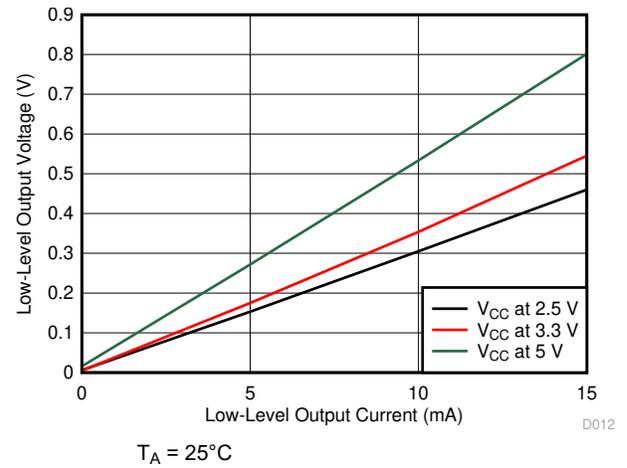
**Figure 5-14. Low-Level Output Voltage vs Low-Level Output Current**
