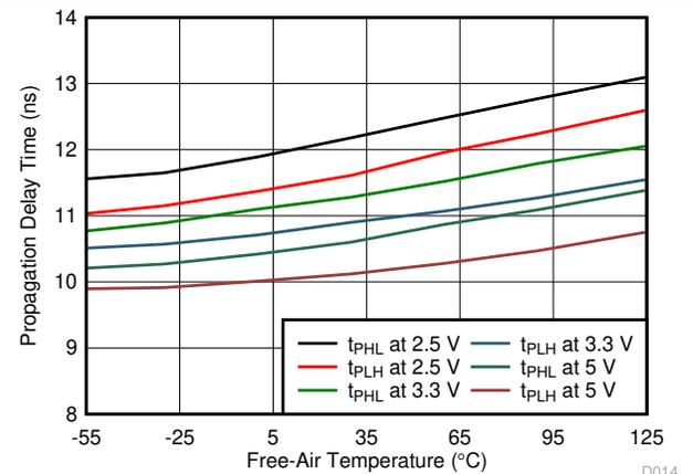
**Figure 5-16. Propagation Delay Time vs Free-Air Temperature**
