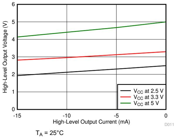
**Figure 5-13. High-Level Output Voltage vs High-level Output Current**
