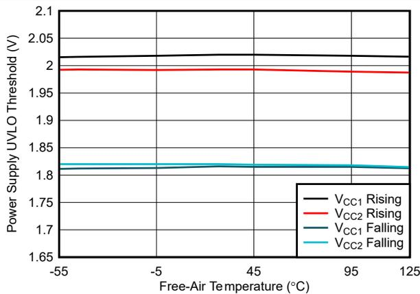
**Figure 5-15. Power Supply Undervoltage Threshold vs Free-Air Temperature**
