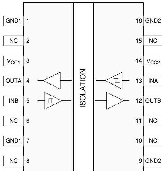
**Figure 5-2. ISO7721 DW Package 16-Pin SOIC Top View**
