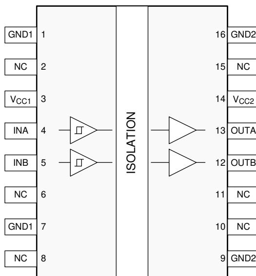
**Figure 5-1. ISO7720 DW Package 16-Pin SOIC Top View**
