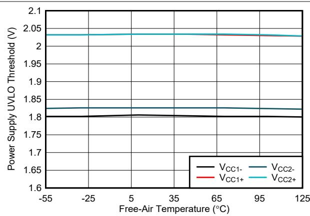
**Figure 6-13. Power Supply Undervoltage Threshold vs Free-Air Temperature**
