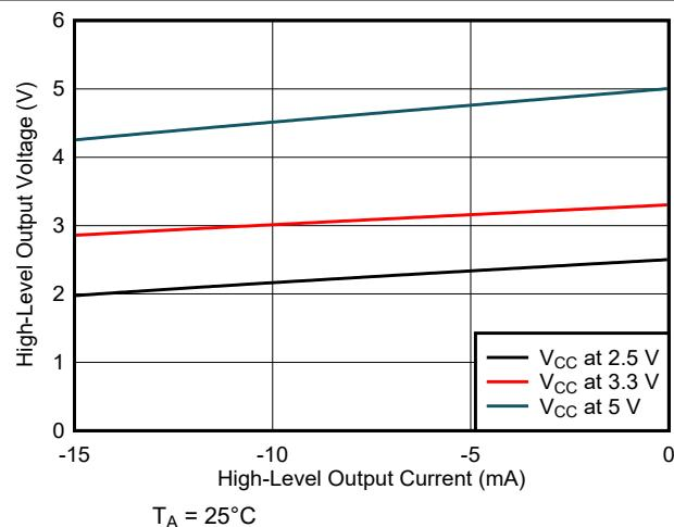
**Figure 6-11. High-Level Output Voltage vs High-level Output Current**
