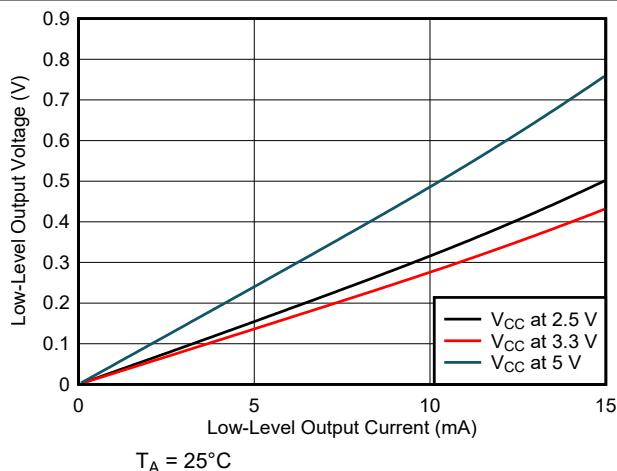
**Figure 6-12. Low-Level Output Voltage vs Low-Level Output Current**
