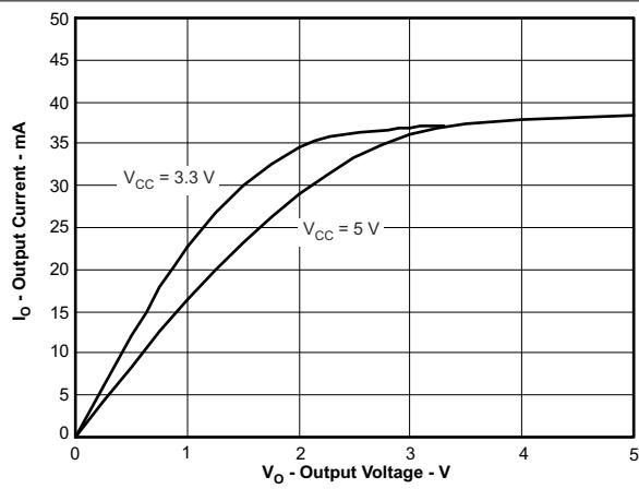
Figure 5-9. Low-Level Output Current vs Low-Level Output Voltage
