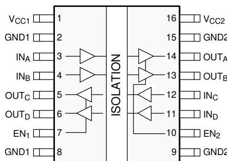
Figure 4-3. ISO7242C-Q1 DW Package 16-Pin SOIC Top View
