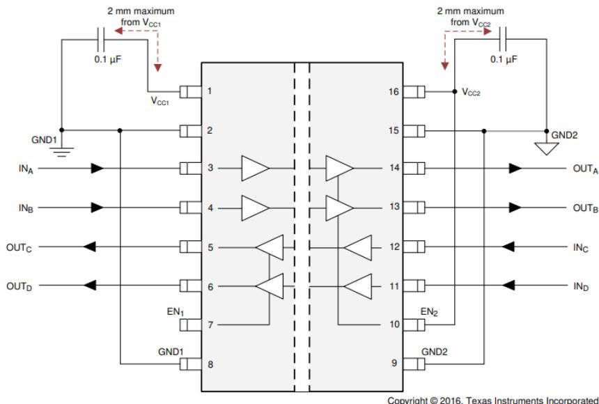
**Figure 8-5. ISO7242x-Q1 Typical Circuit Hook-Up**
