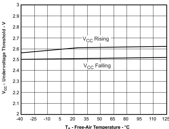
Figure 5-7. V\_cc Failsafe Threshold vs Free-Air Temperature
