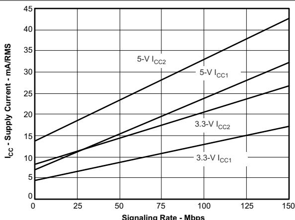
Figure 5-3. ISO7241C RMS Supply Current vs Signaling Rate
