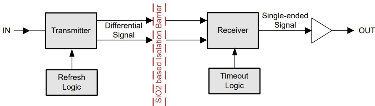
Figure 7-1. Conceptual Block Diagram of a Digital Isolator
