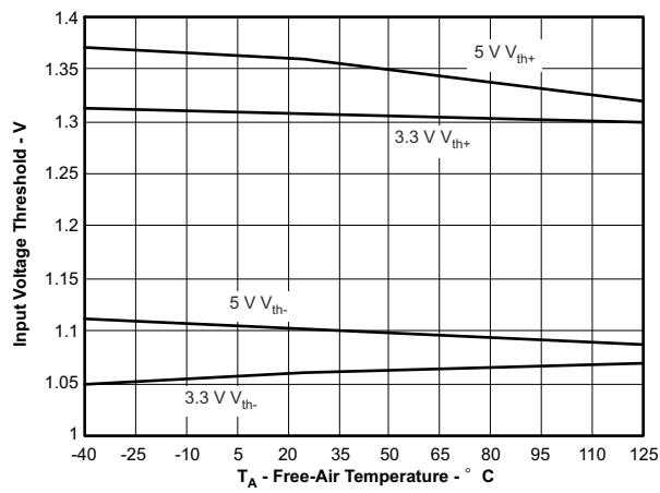
Figure 5-6. Input Voltage Threshold vs Free-Air Temperature
