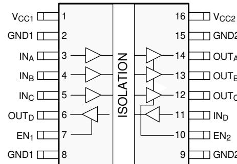
Figure 4-2. ISO7241C-Q1 DW Package 16-Pin SOIC Top View
