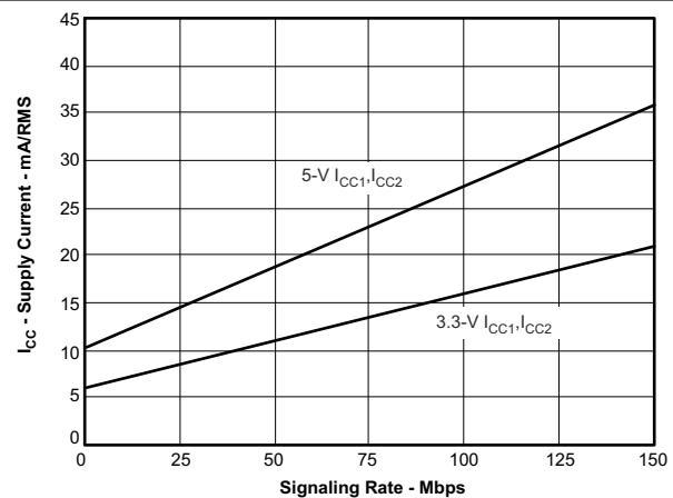
Figure 5-4. ISO7242C RMS Supply Current vs Signaling Rate
