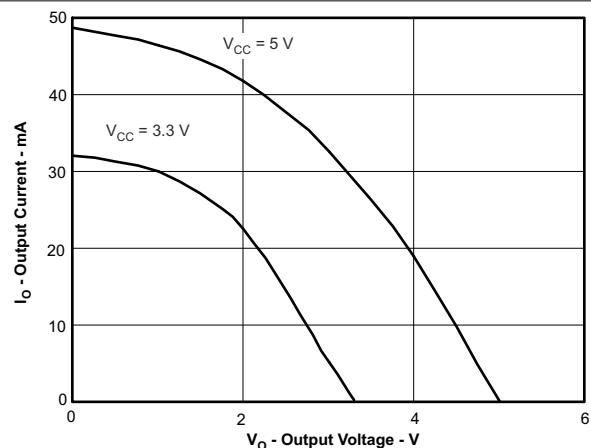
Figure 5-8. High-Level Output Current vs High-Level Output Voltage
