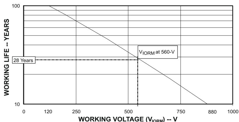
Figure 5-1. Time Dependent Dielectric Breakdown Testing Results
