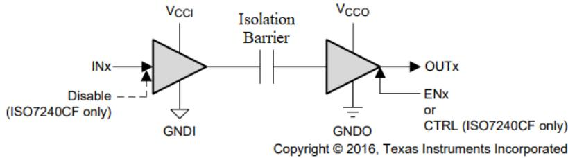
V<sub>CCI</sub> and GNDI are supply and ground connections respectively for the input channels.
