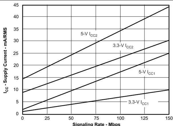
Figure 5-2. ISO7240C RMS Supply Current vs Signaling Rate
