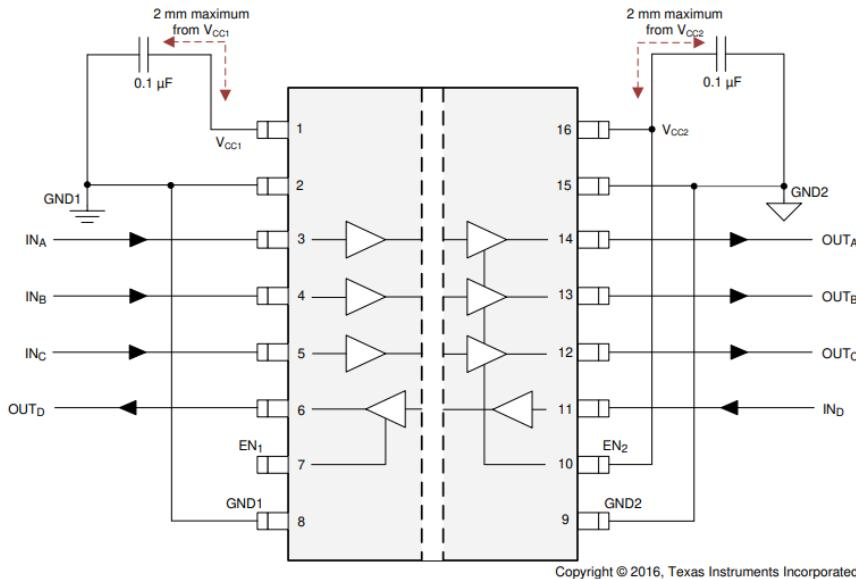
**Figure 8-4. ISO7241x-Q1 Typical Circuit Hook-Up**
