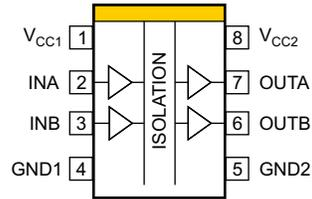
**Figure 4-1. ISO7220x-Q1 D Package 8-Pin SOIC Top View**
