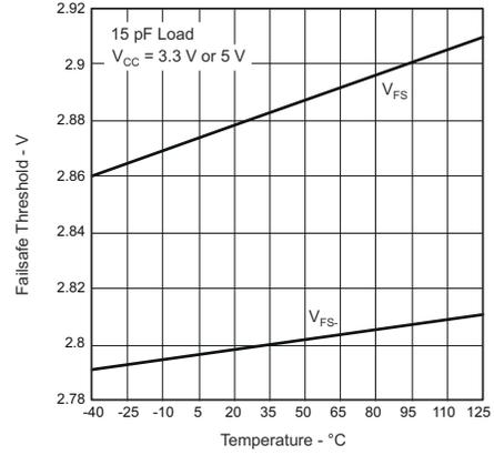
**Figure 5-4. V<sub>CC</sub> Failsafe Threshold vs Free-Air Temperature**
