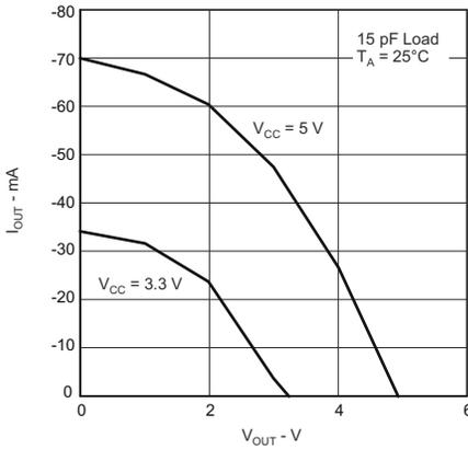
**Figure 5-5. High-Level Output Current vs High-Level Output Voltage**
