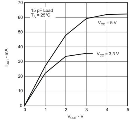
**Figure 5-6. Low-Level Output Current vs Low-Level Output Voltage**
