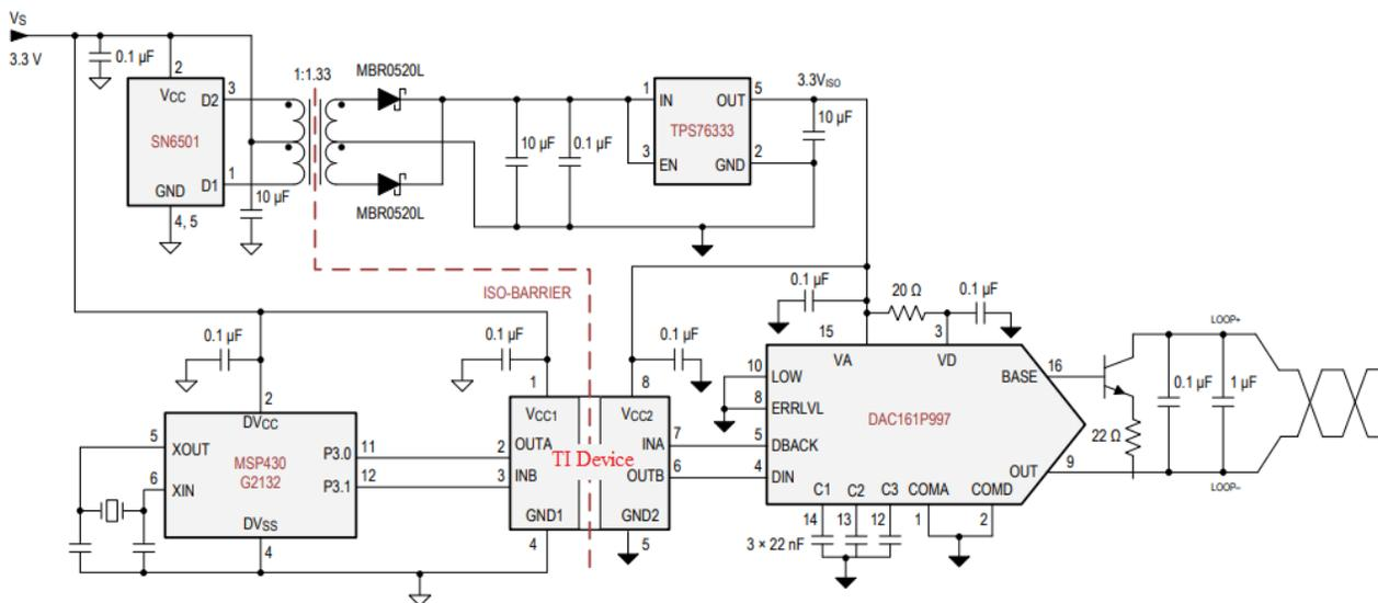
Figure 8-1. Isolated 4- to 20-mA Current Loop
