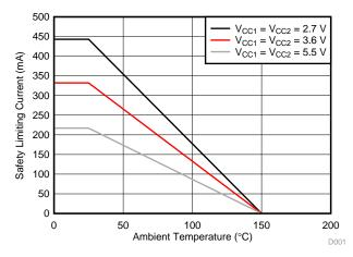
Figure 13. Thermal Derating Curve for Safety Limiting Current per VDE
