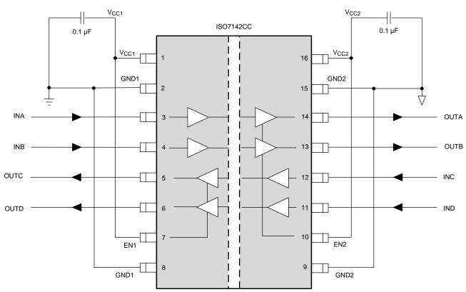
Figure 16. Typical ISO7142CC-Q1 Circuit Hook-up
