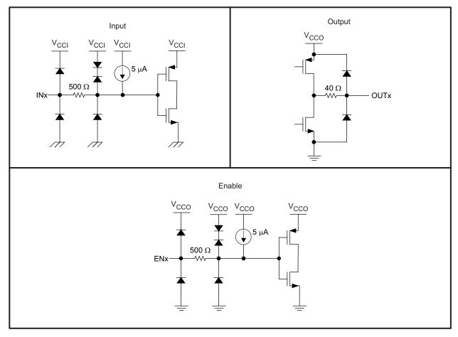
Figure 14. Device I/O Schematics
