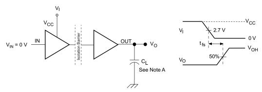
A.  $C_L = 15$  pF and includes instrumentation and fixture capacitance within  $\pm 20\%$ .
