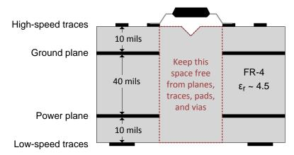
Figure 20. Recommended Layer Stack
