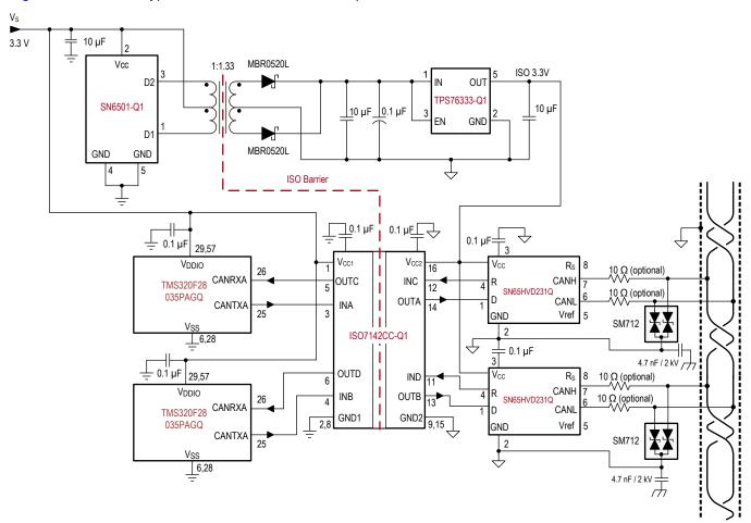
Figure 15. Typical Isolated CAN Application Circuit for ISO7142CC-Q1
