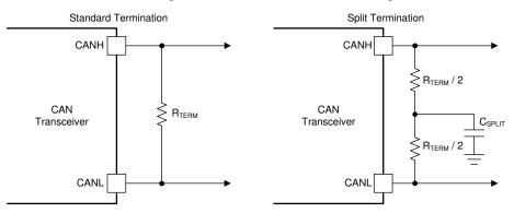
Figure 31. CAN Bus Termination Concepts
