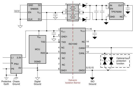
Figure 28. Application Circuit With ISO1042 in 16-SOIC Package
