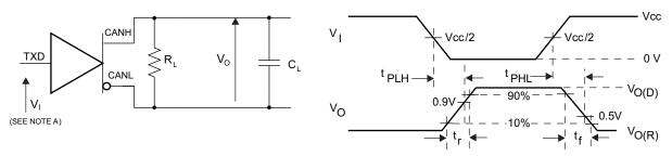
A. The input pulse is supplied by a generator having the following characteristics: PRR  $\leq$  125 kHz, 50% duty cycle,  $t_r \leq 6$  ns,  $t_f \leq 6$  ns,  $Z_O = 50 \Omega$ .
