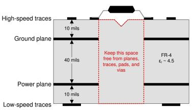
Figure 34. Recommended Layer Stack
