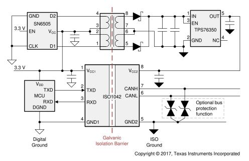
Figure 29. Application Circuit With ISO1042 in 8-SOIC Package
