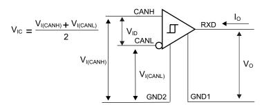
Figure 18. Receiver Voltage and Current Definitions
