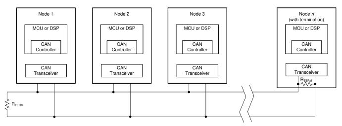
Figure 30. Typical CAN Bus
