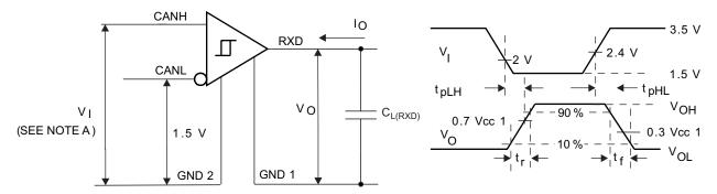
A. The input pulse is supplied by a generator having the following characteristics: PRR  $\leq$  125 kHz, 50% duty cycle,  $t_r \leq 6$  ns,  $t_f \leq 6$  ns,  $Z_O = 50 \Omega$ .
