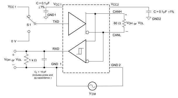
Figure 24. Common-Mode Transient Immunity Test Circuit
