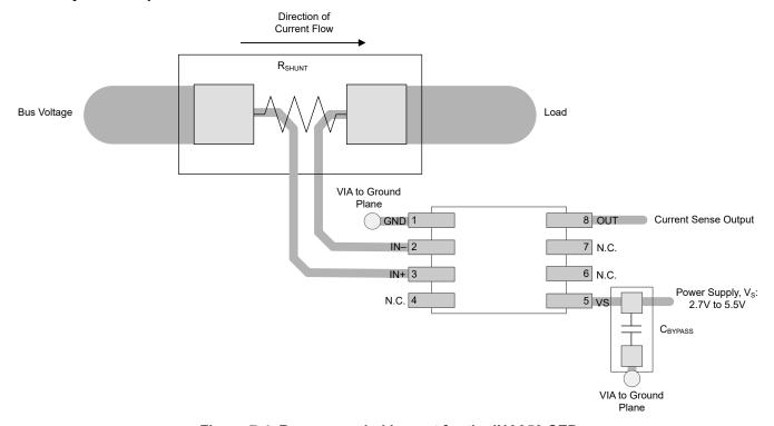
Figure 7-4. Recommended Layout for the INA950-SEP
