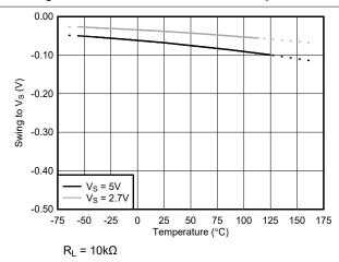
Figure 5-16. Swing to Supply vs. Temperature
