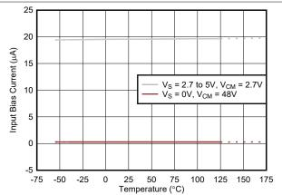
Figure 5-10. Input Bias Current vs. Temperature
