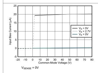
Figure 5-9. Input Bias Current vs. Common-Mode Voltage
