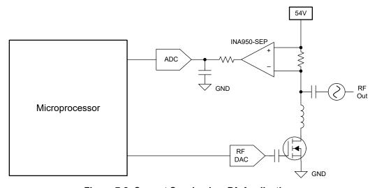
Figure 7-2. Current Sensing in a PA Application
