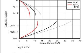
Figure 5-12. Output Voltage vs. Output Current
