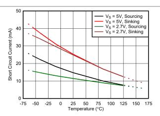
Figure 5-14. Short-Circuit Current vs. Temperature
