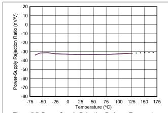
Figure 5-7. Power-Supply Rejection Ratio vs. Temperature
