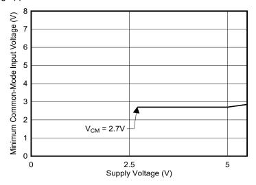
Figure 6-2. Minimum Common-Mode Voltage vs. Supply
