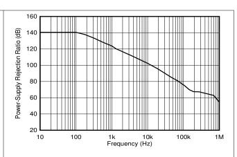
Figure 5-8. Power-Supply Rejection Ratio vs. Frequency
