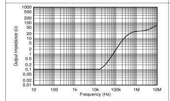
Figure 5-15. Output Impedance vs. Frequency
