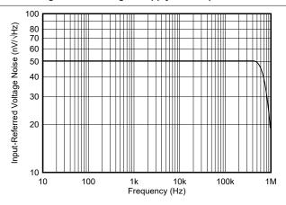
Figure 5-18. Input-Referred Noise vs. Frequency
