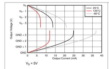
Figure 5-13. Output Voltage vs. Output Current
