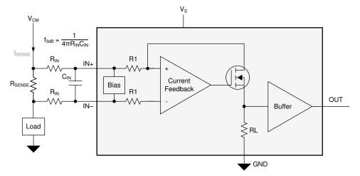
Figure 7-1. Filter at Input Pins
