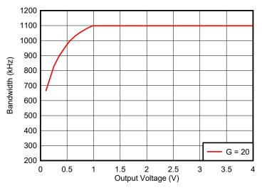
Figure 6-3. Bandwidth vs Output Voltage
