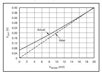
Figure 18. Example for Low V<sub>SENSE</sub> Cases 1 and 3 (Gain = 20)
