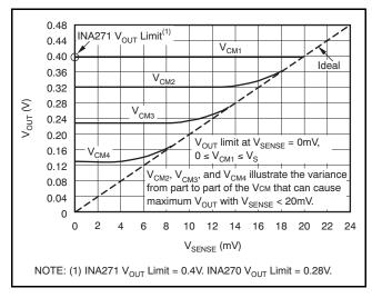
Figure 19. Example for Low  $V_{SENSE}$  Case 2 (Gain = 20)
