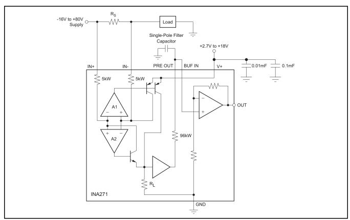
Figure 16. INA271 Basic Connections
