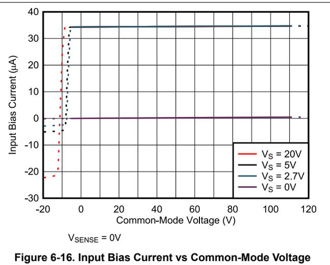
Figure 6-16. Input Bias Current vs Common-Mode Voltage
