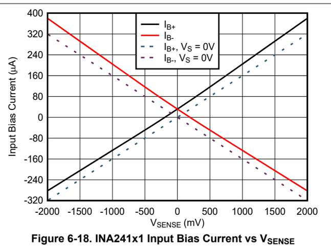
Figure 6-18. INA241x1 Input Bias Current vs  $V_{\text{SENSE}}$
