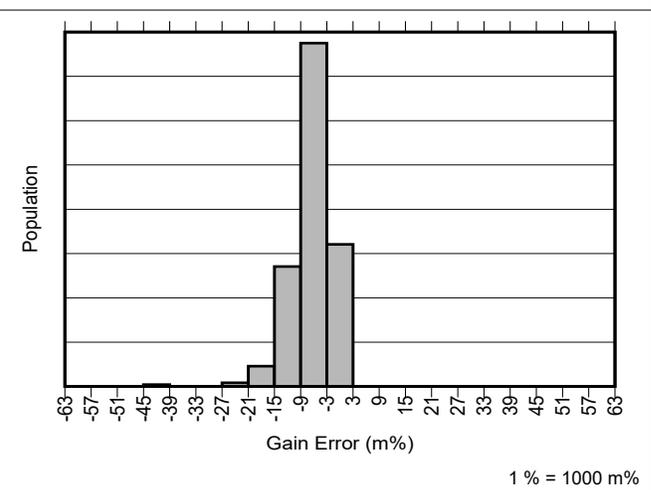
Figure 6-12. All Gains INA241B Gain Error Production Distribution
