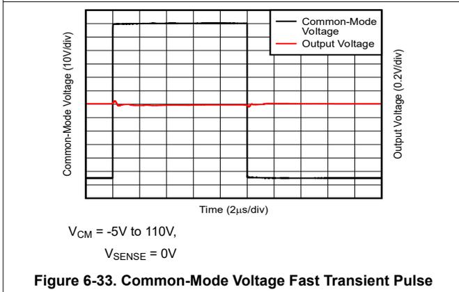
**Figure 6-33. Common-Mode Voltage Fast Transient Pulse**
