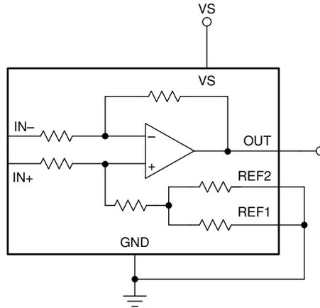
**Figure 7-3. Ground Referenced Output**
