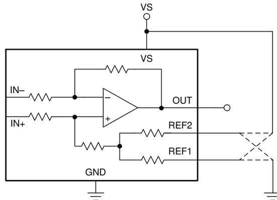
**Figure 7-2. Test Circuit For Reference Divider Accuracy**
