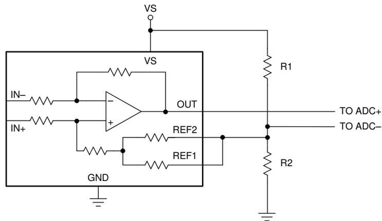
**Figure 7-8. Setting the Reference Using a Resistor Divider**
