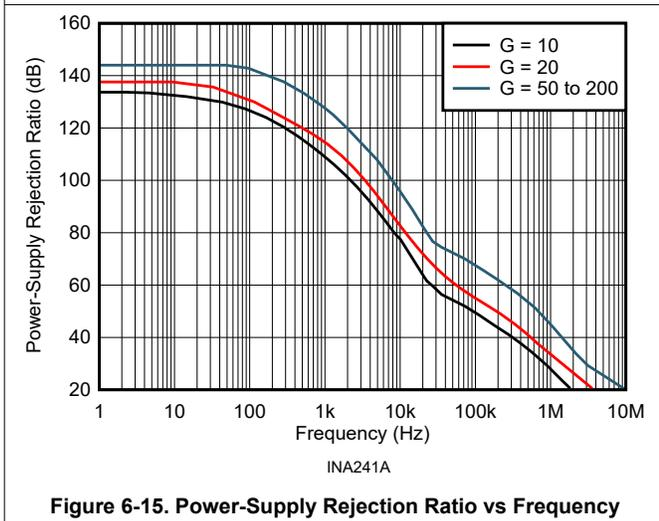
Figure 6-15. Power-Supply Rejection Ratio vs Frequency
