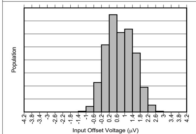
Figure 6-3. INA241A3 and INA241A4 Input Offset Production Distribution
