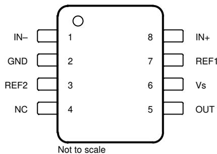
Figure 5-1. INA241x: DDF Package 8-Pin SOT-23 Top View
