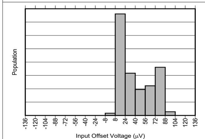
Figure 6-5. All Gains INA241B Input Offset Production Distribution
