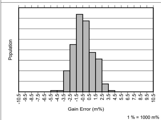
Figure 6-11. INA241A4 and INA241A5 Gain Error Production Distribution
