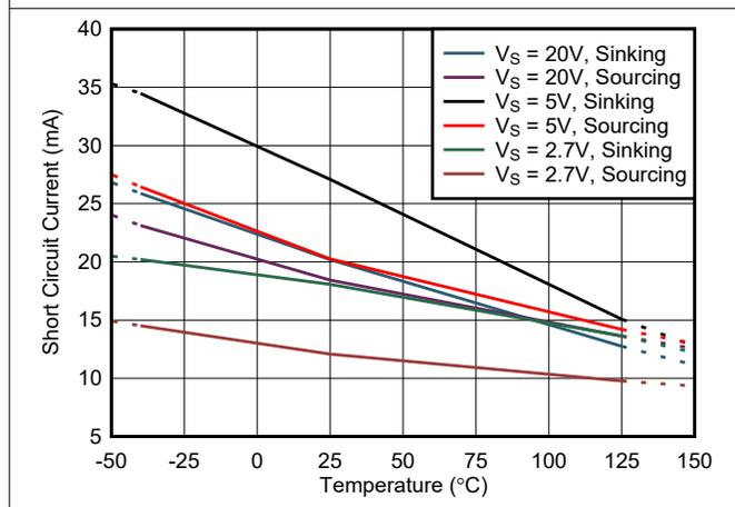
Figure 6-29. Short-Circuit Current vs Temperature
