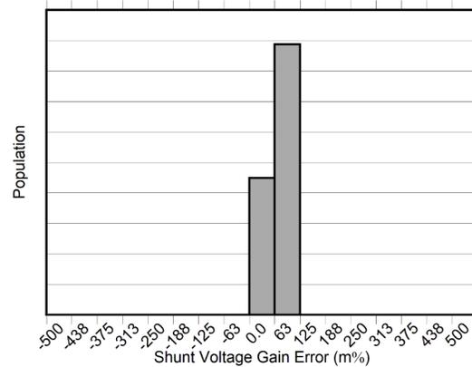
Figure 6-7. Shunt Voltage Gain Error Production Distribution
