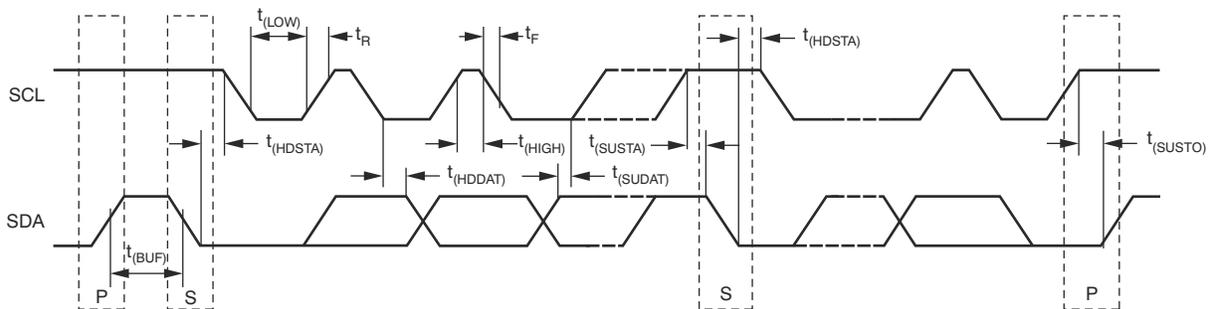
**Figure 6-1. I<sup>2</sup>C Timing Diagram**
