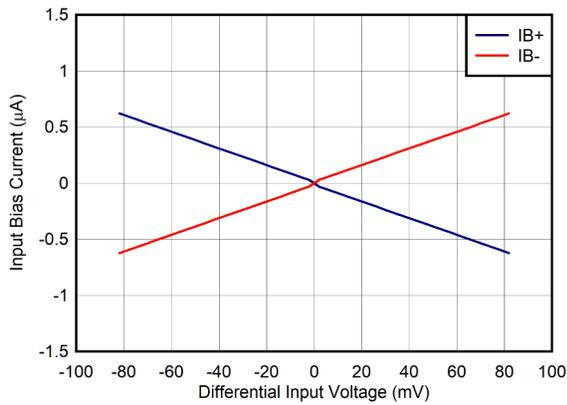
Figure 6-14. Input Bias Current vs Differential Voltage
