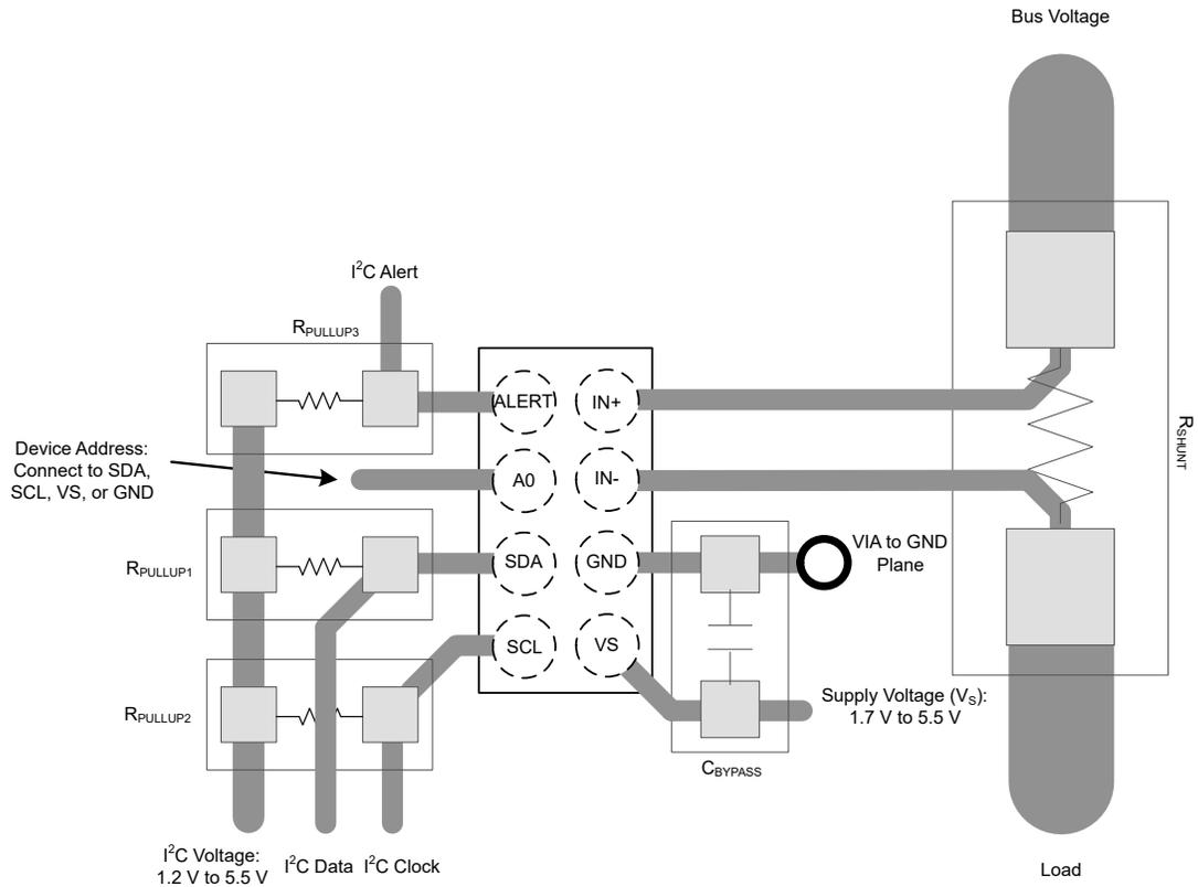
**Figure 8-5. INA234 Layout Example DSBGA (High Side)**
