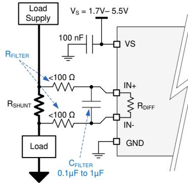
Figure 8-1. Input Filtering
