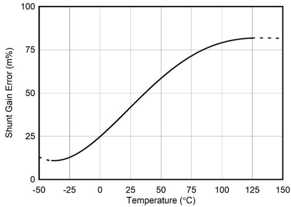
Figure 6-8. Shunt Gain Error vs Temperature
