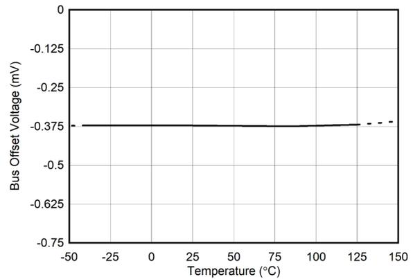
Figure 6-11. Bus Offset Voltage ( $V_{IN-}$ ) vs Temperature
