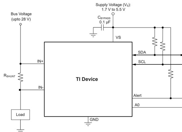
Figure 8-2. Typical High-Side Sensing Circuit Configuration, INA234
