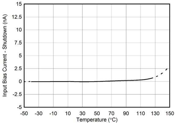
Figure 6-17. Input Bias Current vs Temperature (Shutdown)
