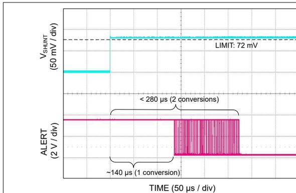
**Figure 8-3. Alert Response ( $t_{CT} = 140 \mu s$ )**
