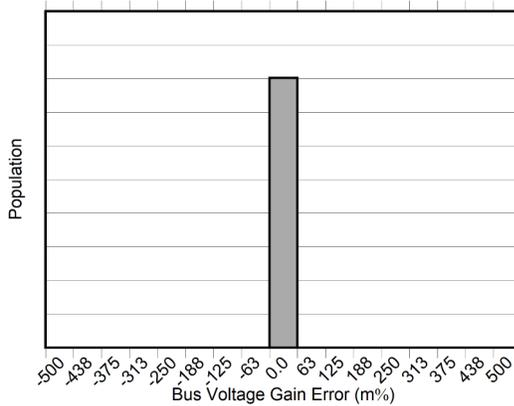
Figure 6-12. Bus Voltage ( $V_{IN-}$ ) Gain Error Production Distribution
