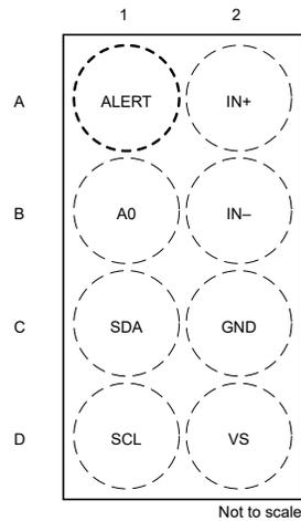
**Figure 5-1. YBJ Package 8-Bump DSBGA (Top View)**
