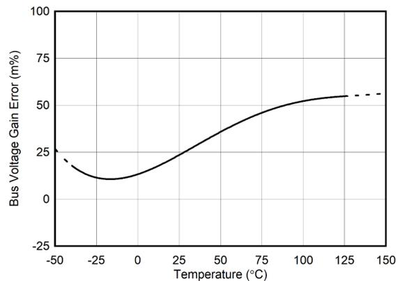
Figure 6-13. Bus Voltage ( $V_{IN-}$ ) Gain Error vs Temperature
