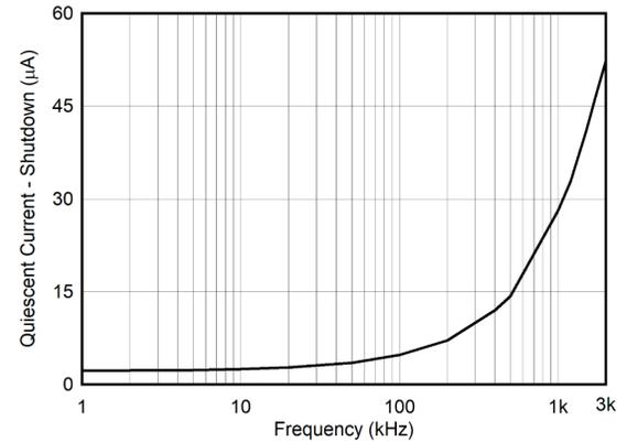
Figure 6-23. Quiescent Current - Shutdown vs SCL Frequency
