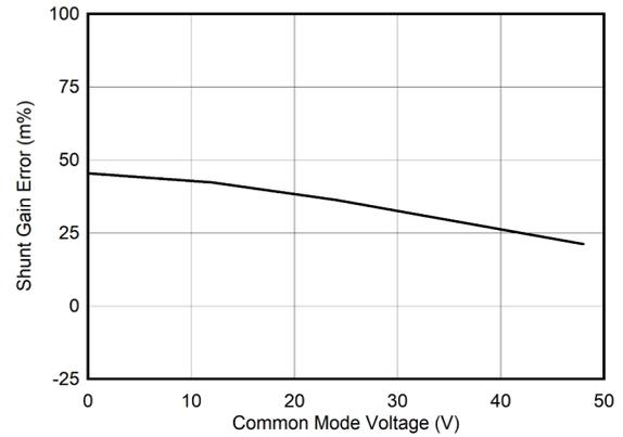
Figure 6-9. Shunt Gain Error vs Common-Mode Voltage
