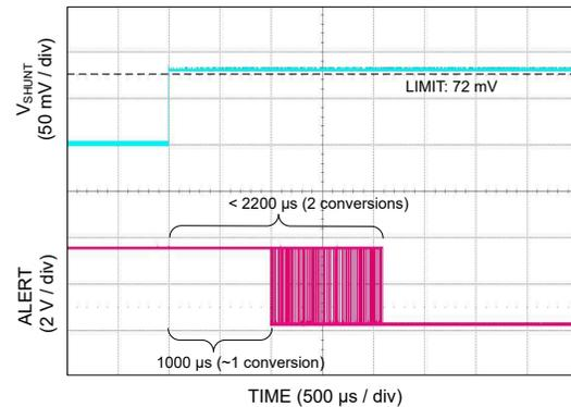
**Figure 8-4. Alert Response ( $t_{CT} = 1.1 ms$ )**
