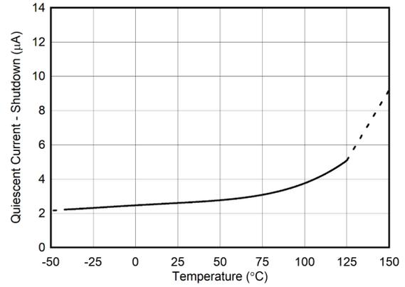
Figure 6-21. Quiescent Current - Shutdown vs Temperature
