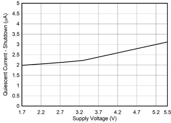
Figure 6-20. Quiescent Current - Shutdown vs Supply Voltage
