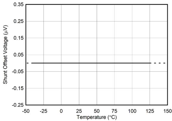
Figure 6-4. Shunt Input Offset Voltage vs Temperature
