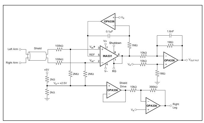
FIGURE 9. Simplified ECG Circuit for Medical Applications.
