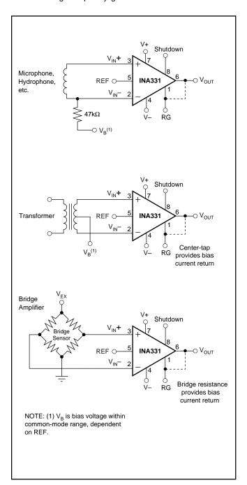
FIGURE 3. Providing an Input Common-Mode Path.
