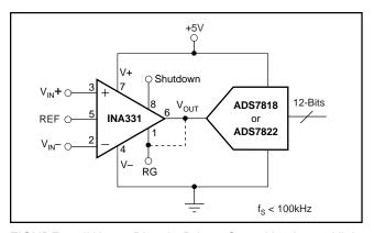
FIGURE 4. INA331 Directly Drives Capacitive-Input, High-Speed A/D Converter.
