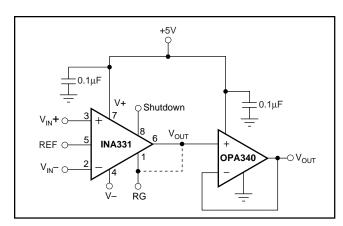
FIGURE 5. Output Buffering Circuit. Able to drive loads as low as  $600\Omega$ .
