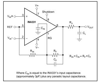
FIGURE 8. Feedback Capacitor Improves Dynamic Perfor-
