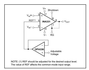
FIGURE 6. Optional Offset Trimming Voltage.
