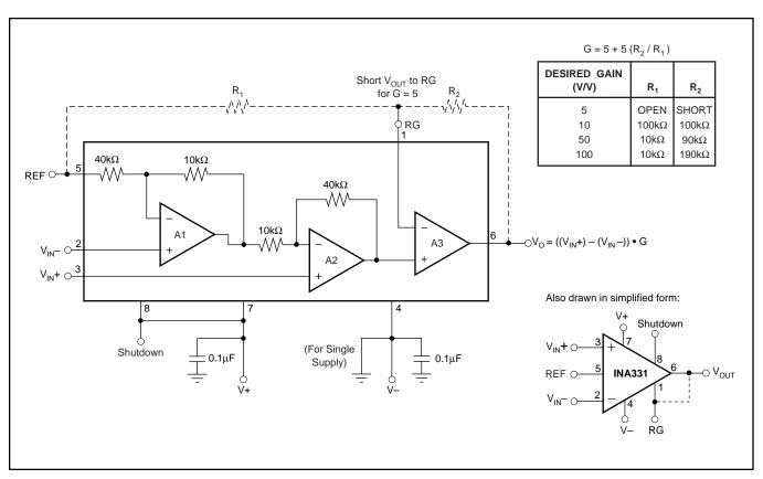
FIGURE 1. Basic Connections.
