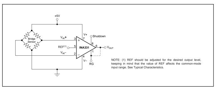
FIGURE 2. Single-Supply Bridge Amplifier.
