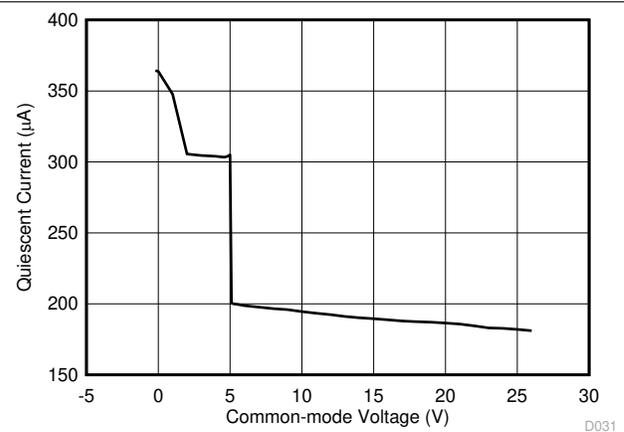
Figure 7-26. Quiescent Current vs. Common-Mode Voltage (INA180-Q1)
