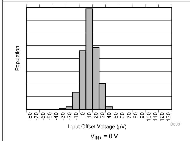
Figure 7-3. Input Offset Voltage Production Distribution A3
