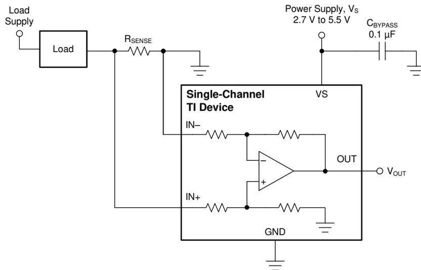
**Figure 9-3. Low-Side Sensing**
