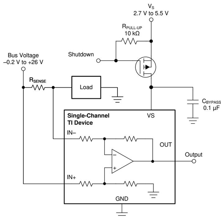
**Figure 8-6. Basic Circuit to Shut Down the INxA180-Q1**
