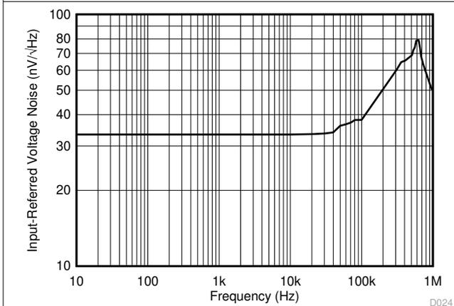
Figure 7-29. Input-Referred Voltage Noise vs. Frequency (A3 Devices)
