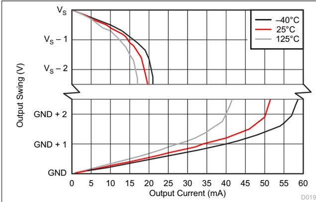
**Figure 7-19. Output Voltage Swing vs. Output Current**
