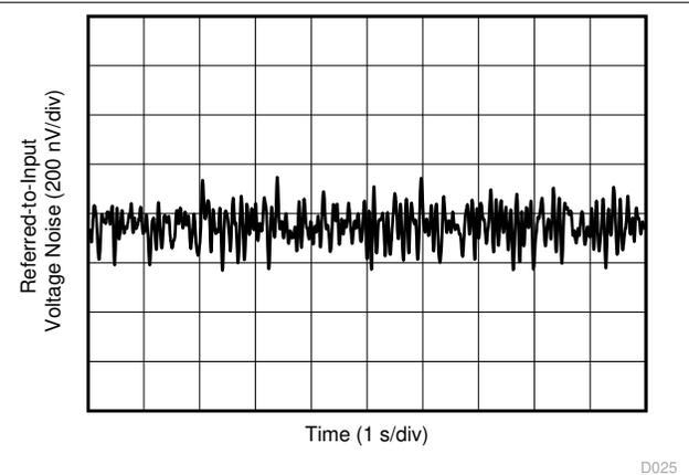
Figure 7-30. 0.1-Hz to 10-Hz Voltage Noise (Referred-to-Input)
