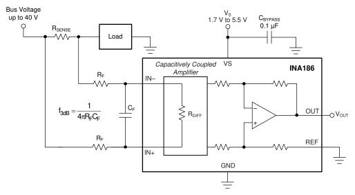
Figure 8-2. Filter at the Input Pins
