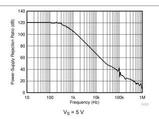
Figure 6-2. Power-Supply Rejection Ratio vs. Frequency
