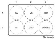
Figure 5-1. DCK Package 6-Pin SC70 Top View
