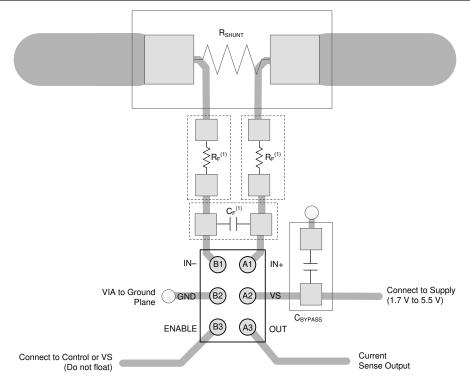
Figure 10-3. Recommended Layout DSBGA (YFD) Package
