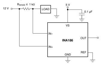
Figure 8-6. Microamp Current Measurement
