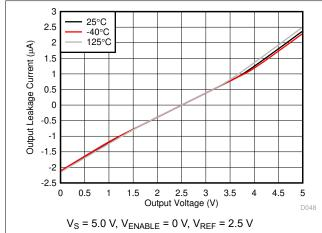
Figure 6-23. Output Leakage vs. Output Voltage (A4 and A5 Devices)
