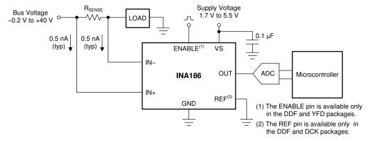
A. To help eliminate ground offset errors between the device and the analog-to-digital converter (ADC), connect the REF pin to the ADC reference input. When driving SAR ADCs, filter or buffer the output of the INA186 before connecting directly to the ADC.
