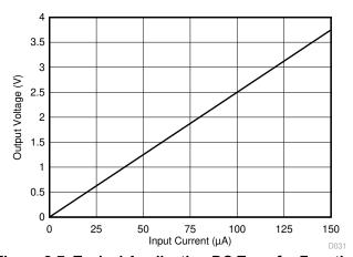
Figure 8-7. Typical Application DC Transfer Function
