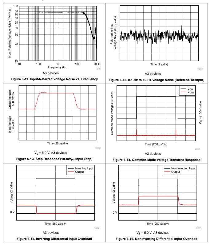
at  $T_A$  = 25°C,  $V_{SENSE}$  =  $V_{IN+}$  –  $V_{IN-}$ ,  $V_S$  = 1.8 V to 5.0 V,  $V_{IN+}$  = 12 V,  $V_{REF}$  =  $V_S$  / 2,  $V_{ENABLE}$  =  $V_S$ , and for all gain options (unless otherwise noted)
