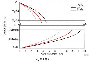
Figure 6-4. Output Voltage Swing vs. Output Current
