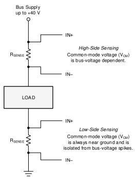
Figure 7-1. High-Side and Low-Side Sensing Connections
