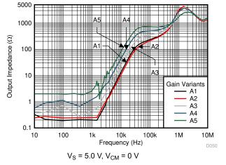
Figure 6-24. Output Impedance vs. Frequency
