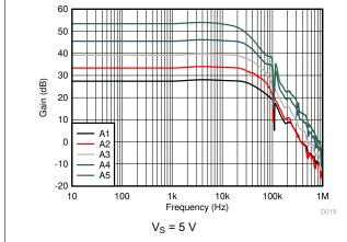
Figure 6-1. Gain vs. Frequency
