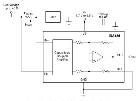
Figure 7-2. Typical Unidirectional Application
