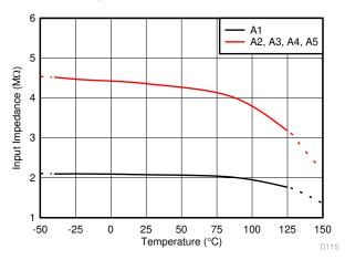
Figure 8-3. Differential Input Impedance vs. Temperature
