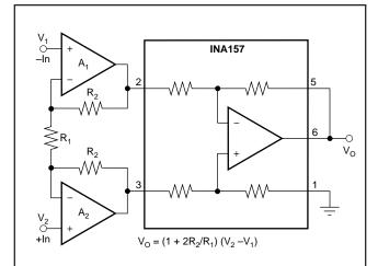
The INA157 can be combined with op amps to form a complete instrumentation amplifier with specialized performance characteristics. Burr-Brown offers many complete high performance IAs. Products with related performances are shown at the right.
