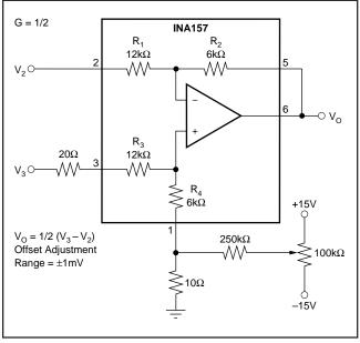
FIGURE 3. Offset Adjustment.
