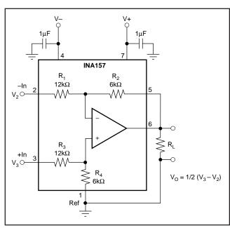
FIGURE 1. G = 1/2 Differential Amplifier (basic power supply and signal connections).
