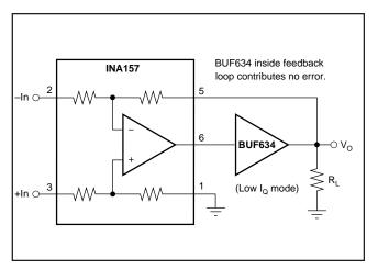
FIGURE 6. Boosting Output Current.
