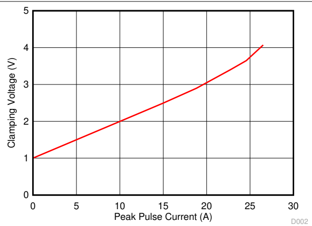
Figure 5-2. Clamping Voltage vs. Peak Pulse Current ( t_p = 8/20\mu s ), GND to Any IO Pin
