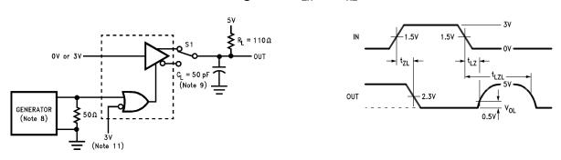
**Note 8:**The input pulse is supplied by a generator having the following characteristics: f = 1.0 MHz, duty cycle = 50%,  $t_f \le 5.0$  ns,  $t_f \le 5.0$  ns, t
