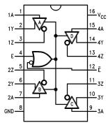
Figure 1. 16-Lead CDIP Package-Top View DS96F172 (See Package Number NFE0016A)
