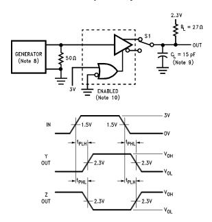
**Note 8:**The input pulse is supplied by a generator having the following characteristics: f = 1.0 MHz, duty cycle = 50%,  $t_f \le 5.0$  ns,  $t_f \le 5.0$  ns, t
