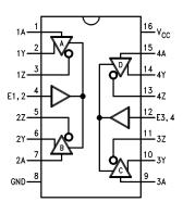
Figure 2. 16-Lead CDIP Package-Top View DS96F174 (See Package Number NFE0016A)
