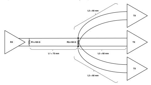
Figure 7-12. FPD-Link Fan-Out Electrical Requirements
