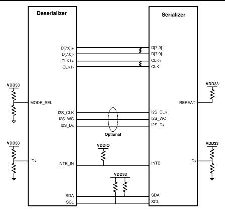
Figure 7-11. HDCP Repeater Connection Diagram
