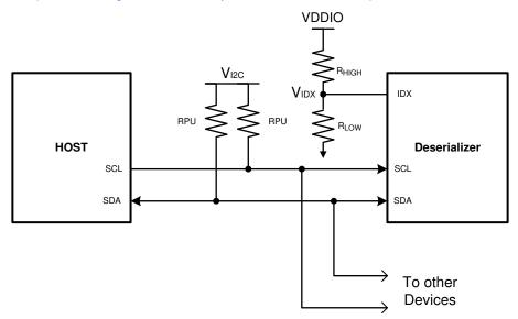
Figure 7-28. Serial Control Bus Connection
