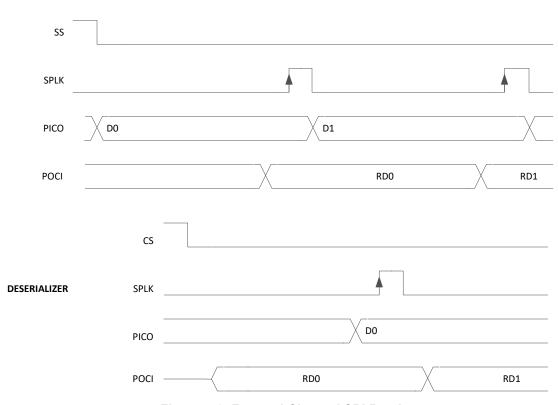
Figure 7-3. Forward Channel SPI Read
