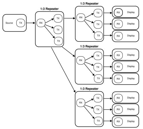
Figure 7-9. HDCP Maximum Repeater Application
