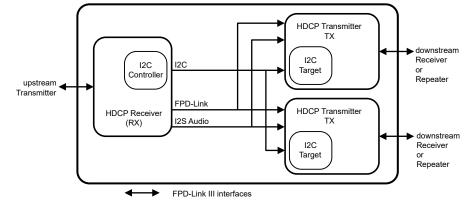
Figure 7-10. HDCP 1:2 Repeater Configuration
