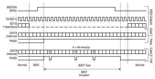
Figure 7-14. BIST Waveforms
