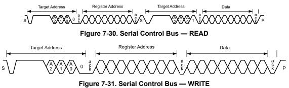
The I2C Controller located in the deserializer must support I2C clock stretching. For more information on I2C interface requirements and throughput considerations, refer to the *I2C Communication Over FPD-Link III with Bidirectional Control Channel* (SNLA131).
