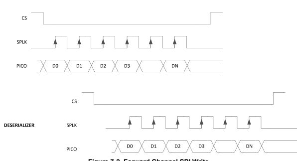
Figure 7-2. Forward Channel SPI Write
