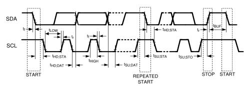
Figure 6-11. Serial Control Bus Timing Diagram
