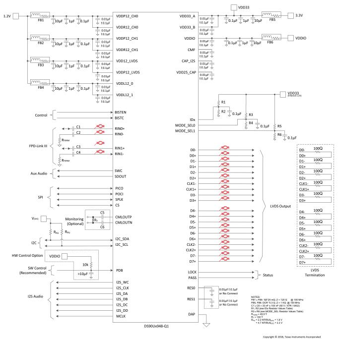
Figure 8-1. Typical Connection Diagram (Coax)
