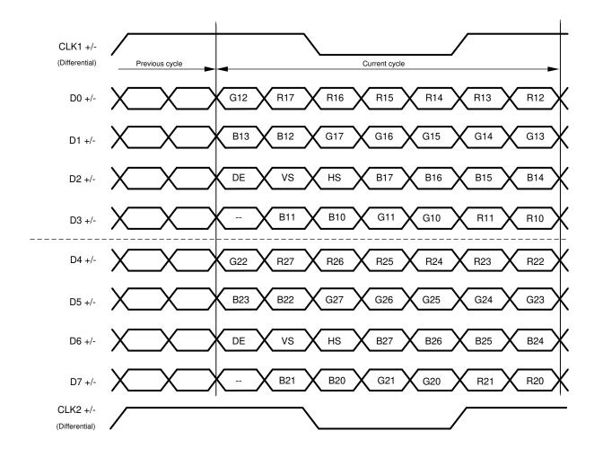
Figure 7-19. 24-Bit Color Dual FPD-Link Mapping: LSBs on D3/D7, "JEIDA" (MAPSEL = L)
