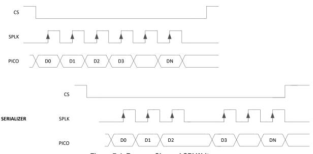
Figure 7-4. Reverse Channel SPI Write
