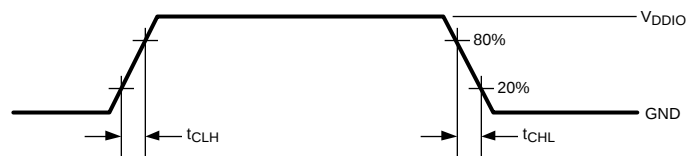
Figure 3. LVCMOS Transition Times
