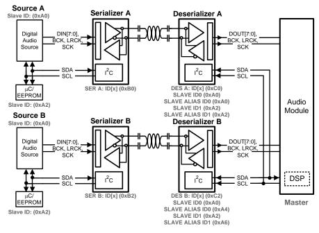
Figure 26. Multiple Device Addressing
