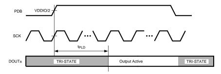
Figure 11. Serializer PLL Lock Time
