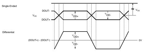
Figure 8. Serializer VOD and Differential Diagram
