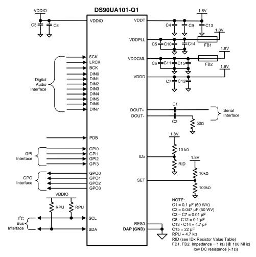
Figure 32. DS90UA101-Q1 Typical Connection Diagram (Coaxial Interconnect)
