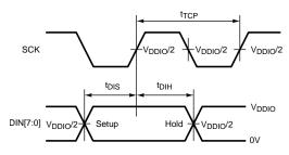
Figure 10. Serializer Setup/Hold Times
