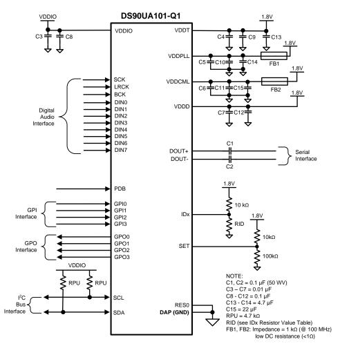
Figure 33. DS90UA101-Q1 Typical Connection Diagram (STP Interconnect)
