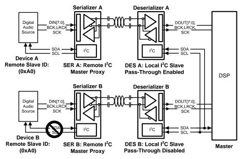
Figure 25. I<sup>2</sup>C Pass-Through
