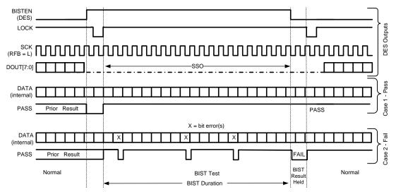
Figure 29. BIST Timing Diagram
