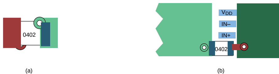
Figure 21. Typical Decoupling Capacitor Layouts
