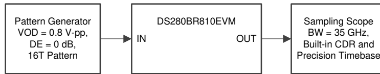
Figure 23. FIR Test Setup
