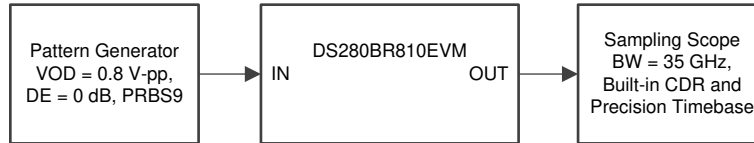
Figure 11. Minimal Rx/Tx Channel Test Setup
