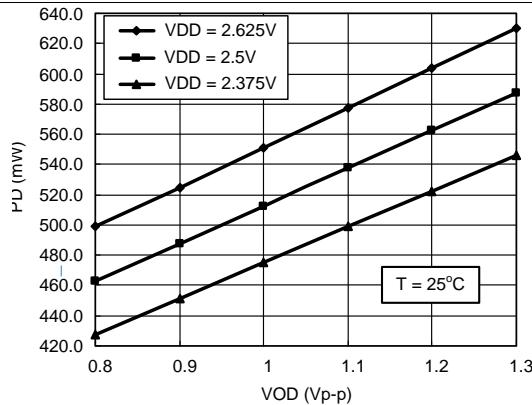
**Figure 5. Typical Power Dissipation vs. Output Voltage Amplitude Setting**
