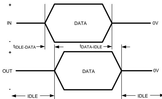
**Figure 3. Transmit Idle-Data and Data-Idle Response Time**
