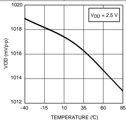
**Figure 7. Channel-B Output Differential Voltage Vs. Temperature (VOD = 1000 mV setting)**
