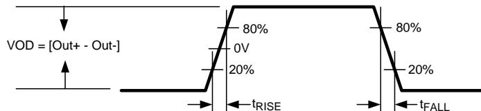
Figure 1. Output and Rise And Fall Transition Time
