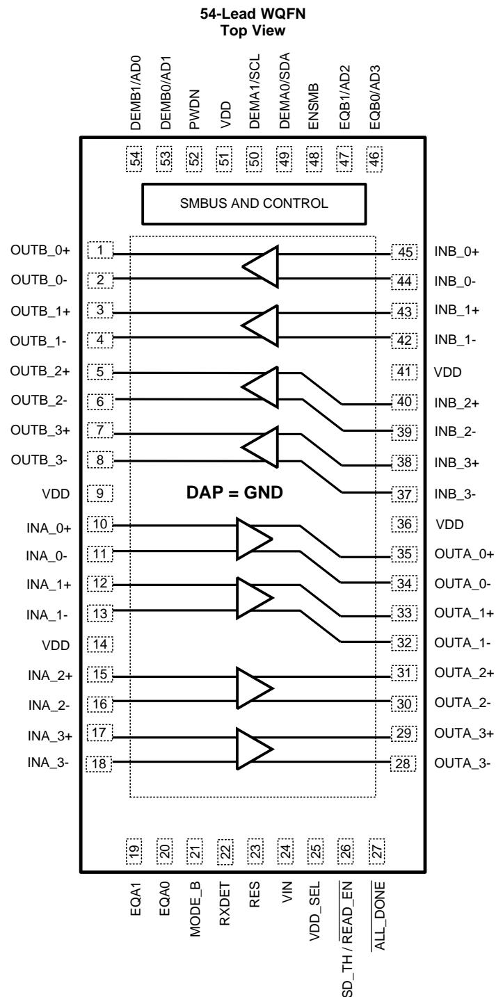
NOTE: Above 54-lead WQFN graphic is a TOP VIEW, looking down through the package.
