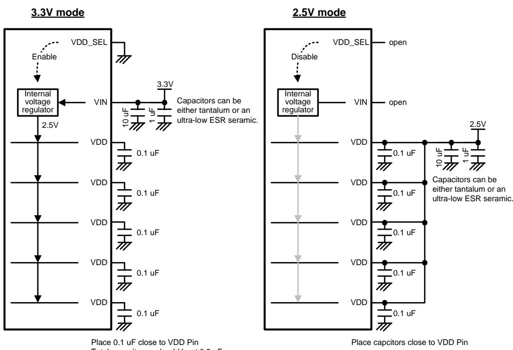
**Figure 21. 3.3V or 2.5V Supply Connection Diagram**
