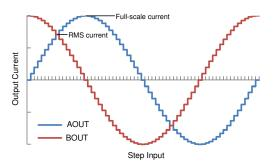
Figure 12. Full-Scale and rms Current
