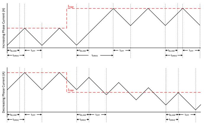
Figure 20. Fast/Fast Decay Mode
