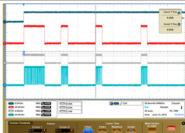
Figure 8-9. ITRIP Across TOFF and Load Current
