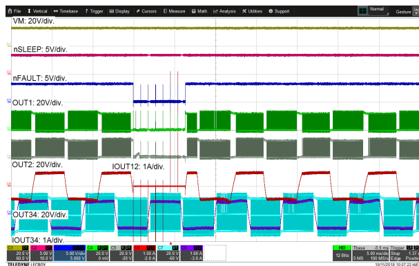
Figure 8-15. Over Current Protection and Recovery
