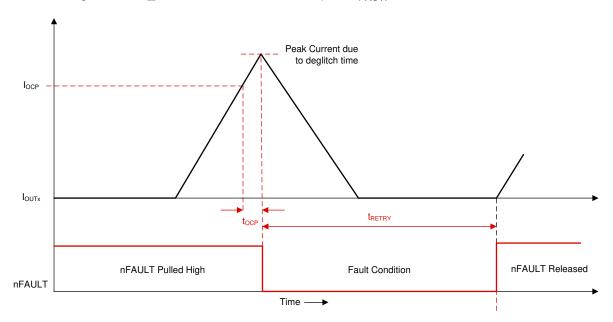
Figure 7-38. Overcurrent Protection - Automatic Retry Mode
