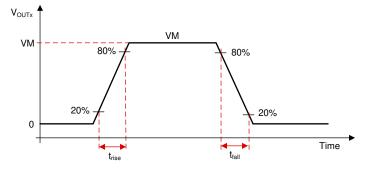
Figure 7-11. Slew Rate Timings
