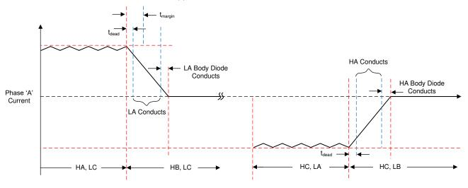
Figure 7-25. Current Waveforms for ASR in BLDC Motor Commutation
