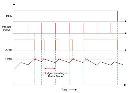
Figure 7-34. Cycle-by-Cycle Current-Limit Operation with 100% PWM Duty Cycle
