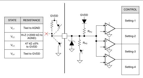
Figure 7-19. Four Level Input Pin Structure
