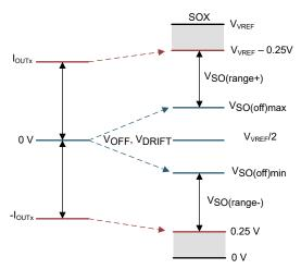
Figure 7-21. Bidirectional Current Sense Output
