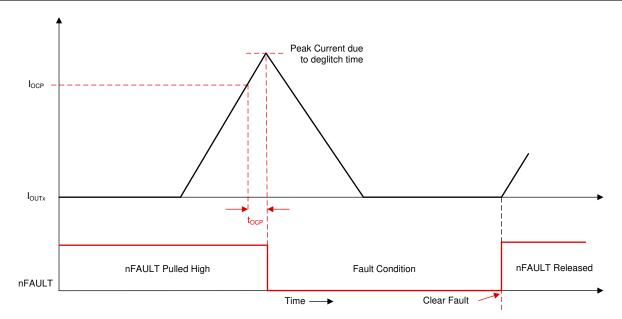
Figure 7-37. Overcurrent Protection - Latched Shutdown Mode
