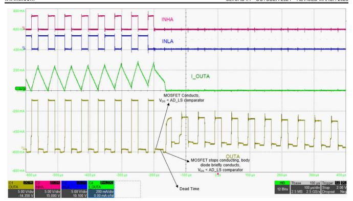
Figure 9-3. Active demagnetization enabled in DRV8376
