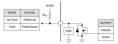
Figure 7-17. Open Drain
