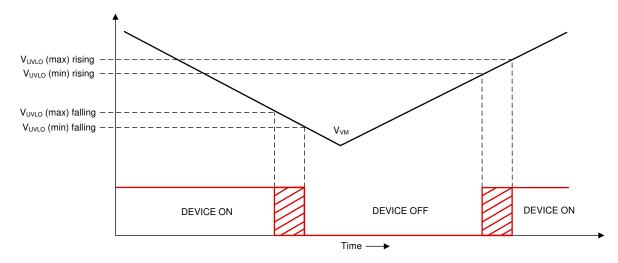
Figure 7-35. VM Supply Undervoltage Lockout
