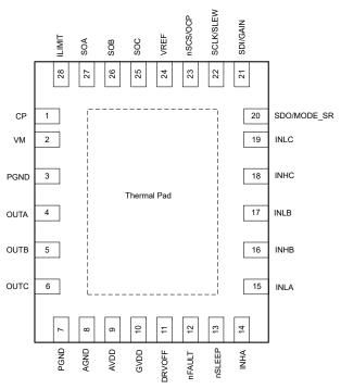
Figure 5-1. DRV8376 28-Pin VQFN With Exposed Thermal Pad Top View
