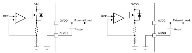
Figure 7-7. GVDD Linear Regulator Block Diagram Figure 7-8. AVDD Linear Regulator Block Diagram
