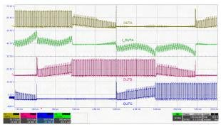
Figure 9-7. Driver PWM with Active Demagnetization Disabled
