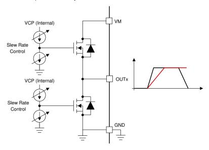
Figure 7-10. Slew Rate Circuit Implementation
