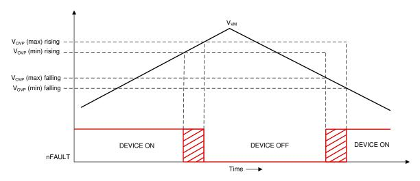
Figure 7-36. Over Voltage Protection
