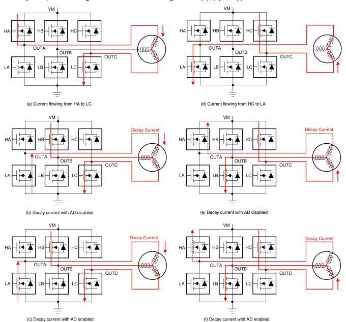
Figure 7-24. ASR in BLDC Motor Commutation
