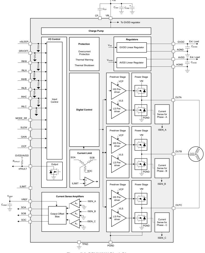
Figure 7-2. DRV8376H Block Diagram
