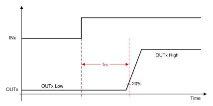
Figure 7-14. Propagation Delay Timing
