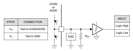
Figure 7-15. Logic-Level Input Pin Structure
