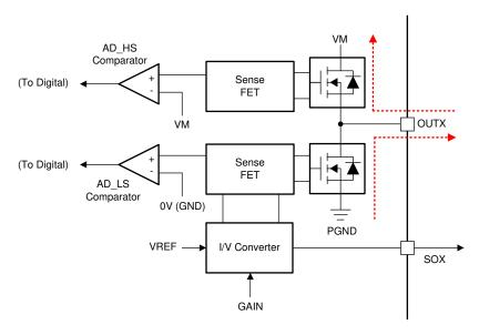
Figure 7-23. Active Demagnetization Operation
