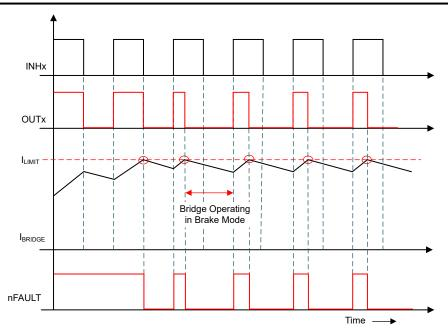
Figure 7-29. Cycle-by-Cycle Current-Limit Operation
