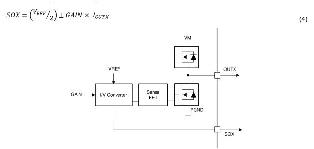
Figure 7-20. Integrated Current Sense Amplifier
