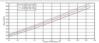
Figure 6-3.  $R_{\text{DS(ON)}}$  (high and low side combined) for MOSFETs over temperature
