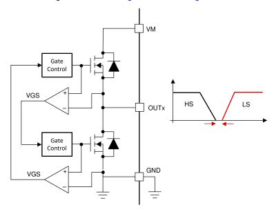
Figure 7-12. Cross Conduction Protection
