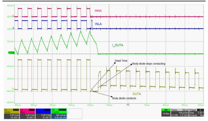
Figure 9-2. Active demagnetization disabled in DRV8376
