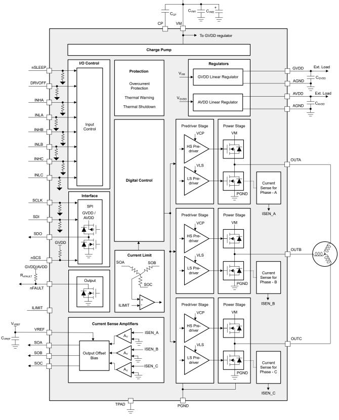
Figure 7-1. DRV8376S Block Diagram
