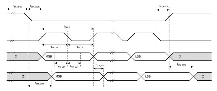
Figure 6-1. SPI Secondary Mode Timings
