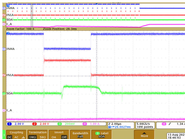
Figure 9-6. Driver PWM operation with feedback
