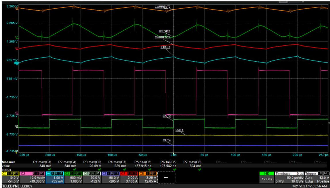
Figure 7-3. Dual H-bridge Operation, VM = 24 V
