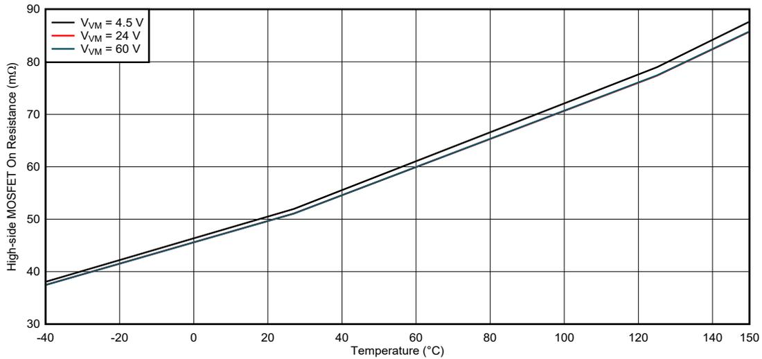
**Figure 5-5. High-side FET on Resistance, Dual H-bridge Mode**
