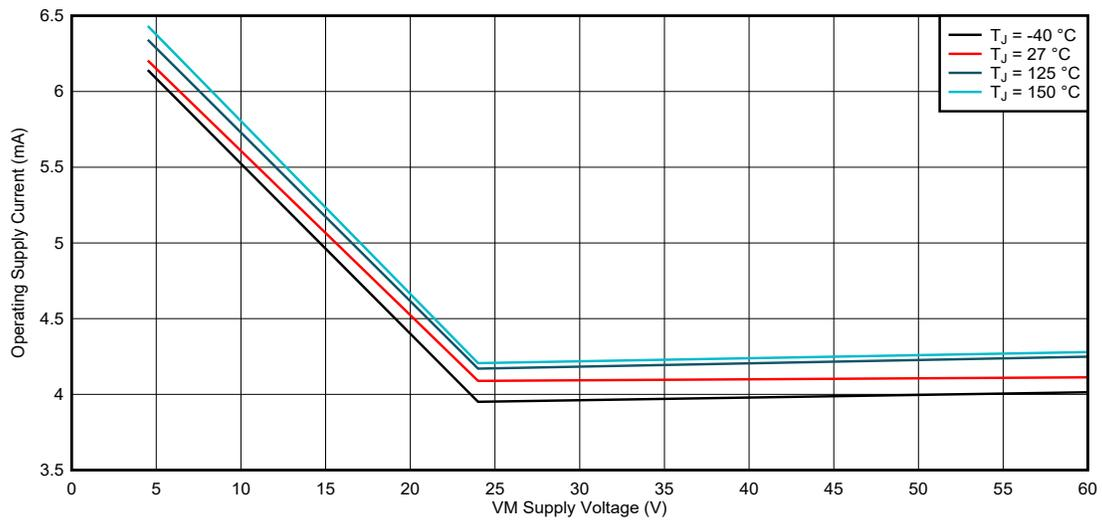
Figure 5-3. Operating Supply Current, VCC = External 5 V
