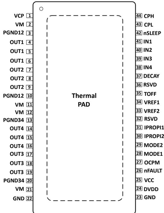
Figure 4-2. Dual H-bridge Mode, Top View
