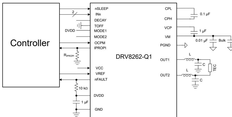
**Figure 7-7. Driving one TEC with higher current**
