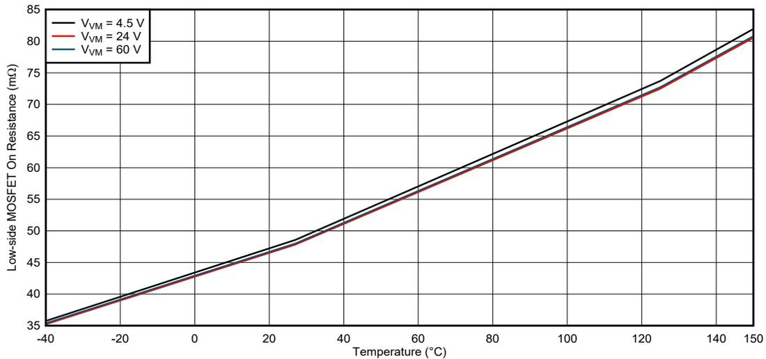
**Figure 5-6. Low-side FET on Resistance, Dual H-bridge Mode**
