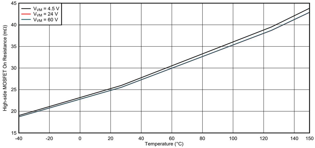
Figure 5-7. High-side FET on Resistance, Single H-bridge Mode
