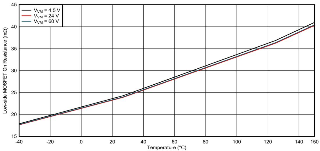
Figure 5-8. Low-side FET on Resistance, Single H-bridge Mode
