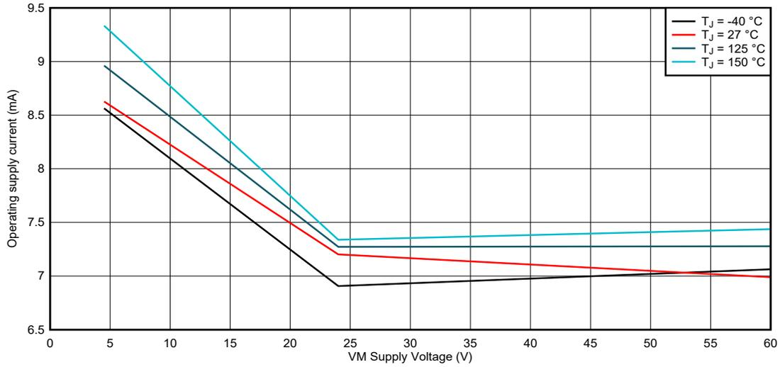
**Figure 5-4. Operating Supply Current, VCC = DVDD**
