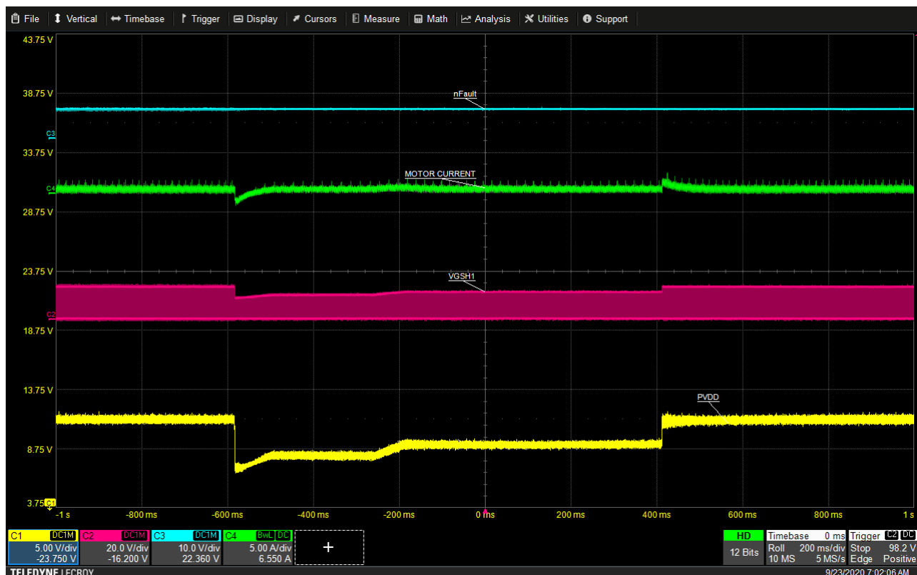
Figure 8-4. Driver PWM Operation During Warm Crank Pulse
