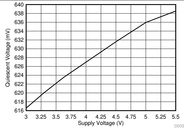
Figure 2. Quiescent Voltage vs Supply Voltage
