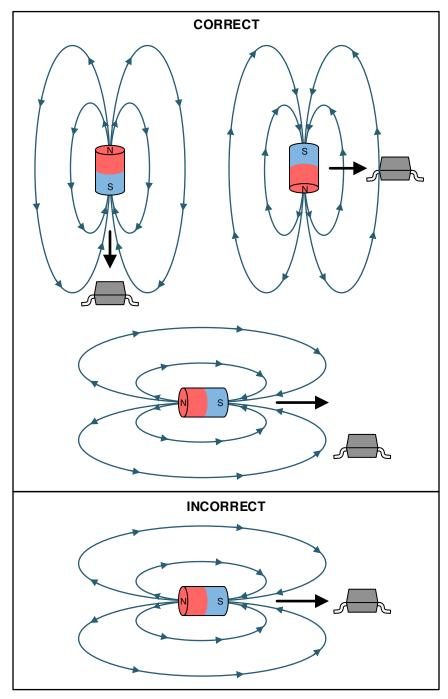
**Figure 8-4. Correct and Incorrect Magnet Approaches**
