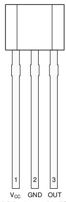
Figure 5-2. LPG Package 3-Pin TO-92 Top View
