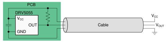
Figure 8-1. Wire Fault Detection Circuit
