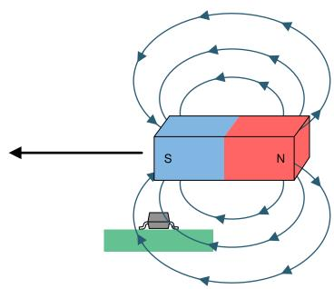
Figure 8-2. Common Magnet Orientation
