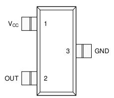
Figure 5-1. DBZ Package 3-Pin SOT-23 Top View
