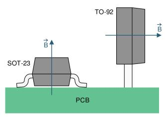
Figure 7-1. Direction of Sensitivity
