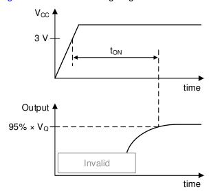
Figure 7-4. t<sub>ON</sub> Definition
