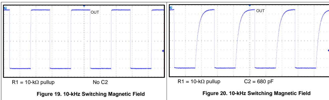
Figure 19. 10-kHz Switching Magnetic Field
