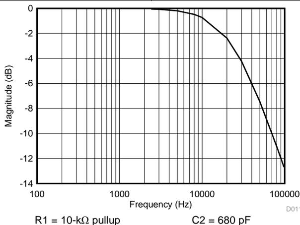
Figure 21. Low-Pass Filtering
