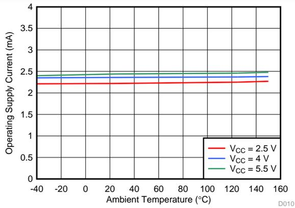
Figure 10.  $I_{CC}$  vs Temperature (DRV5015A2-Q1, DRV5015A3-Q1)
