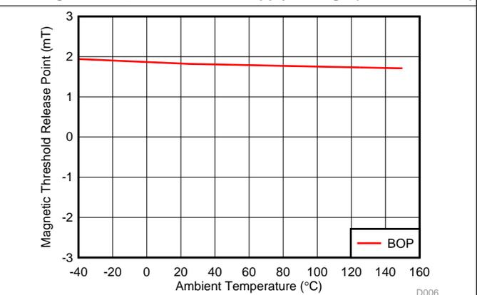
Figure 6.  $B_{OP}$  Threshold vs Temperature (DRV5015A2-Q1, DRV5015A3-Q1)
