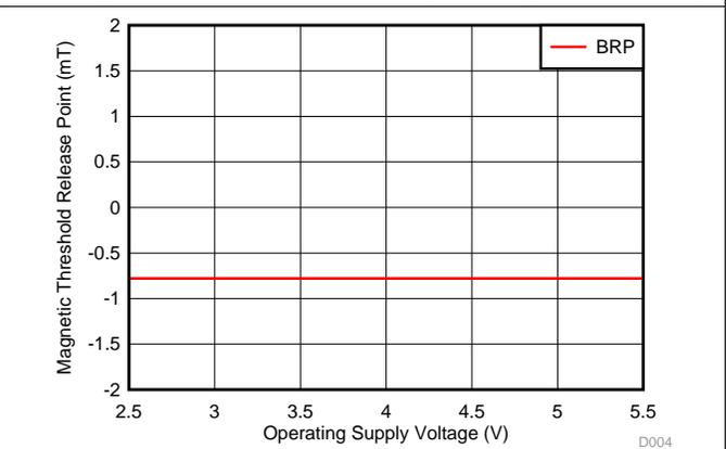
Figure 4.  $B_{RP}$  Threshold vs Supply Voltage (DRV5015A1-Q1)
