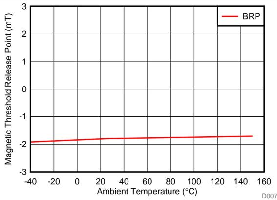
Figure 7.  $B_{RP}$  Threshold vs Temperature (DRV5015A2-Q1, DRV5015A3-Q1)
