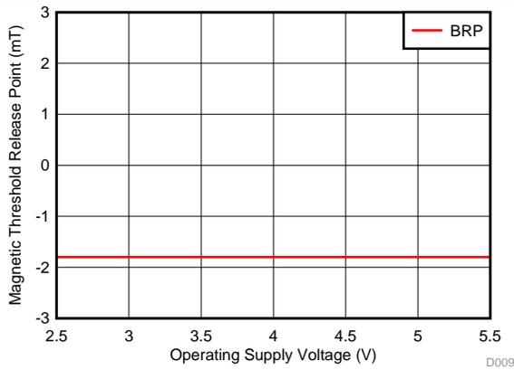
Figure 9.  $B_{RP}$  Threshold vs Supply Voltage (DRV5015A2-Q1, DRV5015A3-Q1)
