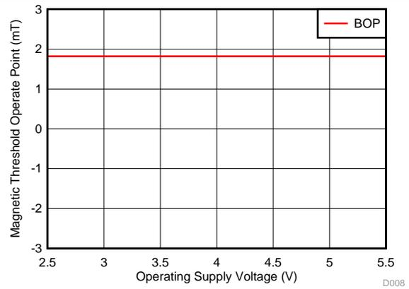
Figure 8.  $B_{OP}$  Threshold vs Supply Voltage (DRV5015A2-Q1, DRV5015A3-Q1)
