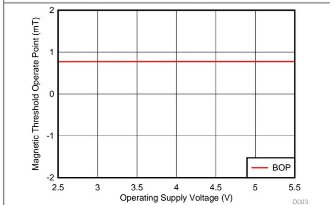
Figure 3.  $B_{OP}$  Threshold vs Supply Voltage (DRV5015A1-Q1)
