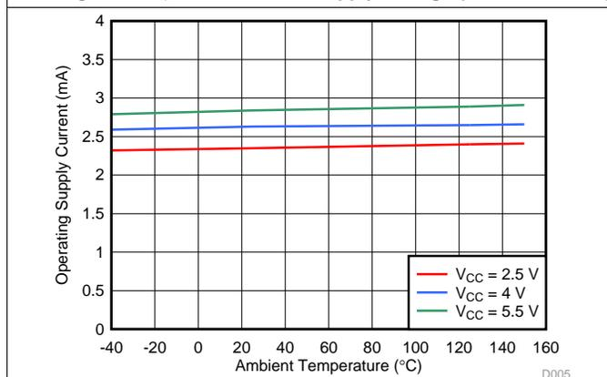
Figure 5.  $I_{CC}$  vs Temperature (DRV5015A1-Q1)
