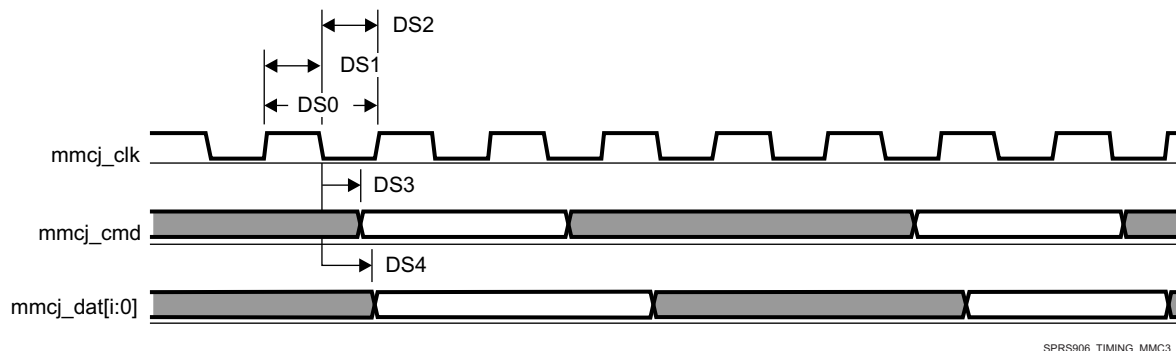
Figure 5-100. MMC/SD/SDIOj in - Default Speed - Transmitter Mode
