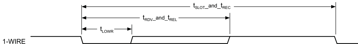
Figure 5-51. 1-Wire—Read Bit (Data)
