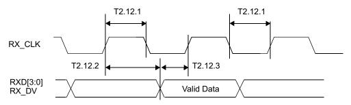
Figure 4-12. 10 Mb/s MII Receive Timing
