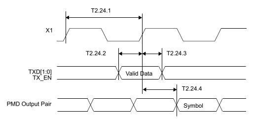
Figure 4-27. RMII Transmit Timing
