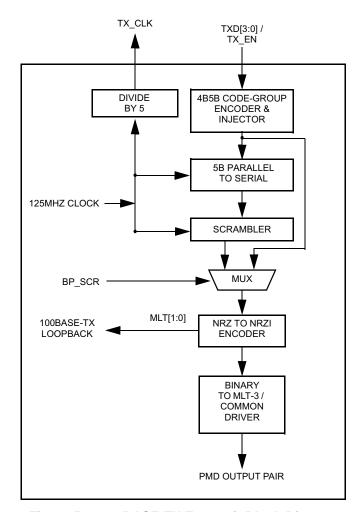
Figure 5-6. 100BASE-TX Transmit Block Diagram
