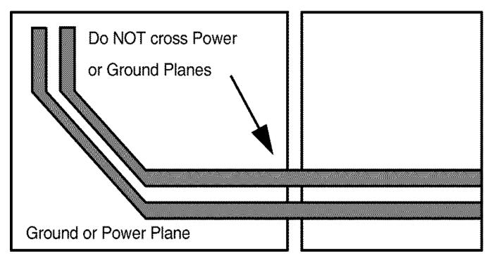
Figure 8-2. Differential Signal Pair-Plane Crossing
