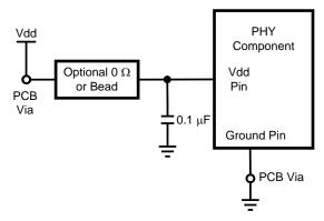
Figure 7-1. V<sub>DD</sub> Bypass Layout
