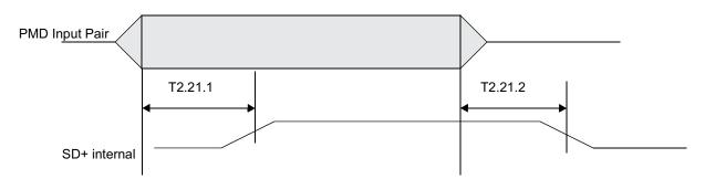
Figure 4-24. 100BASE-TX Signal Detect Timing
