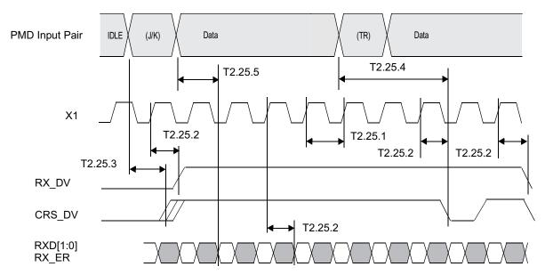
Figure 4-28. RMII Receive Timing
