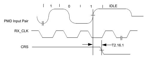
Figure 4-19. 10BASE-T Receive Timing (End of Packet)
