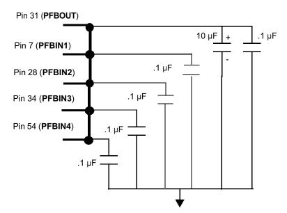
Figure 6-3. Power Feedback Connections
