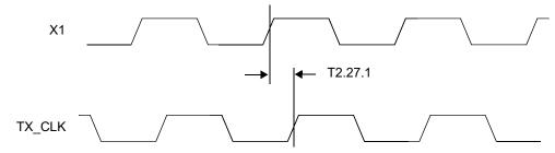
Figure 4-33. 100 Mb/s X1 to TX\_CLK Timing
