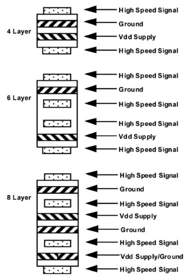
Figure 8-3. PCB Stripline Layer Stacking
