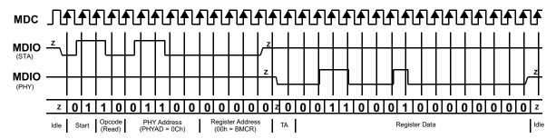
Figure 5-2. Typical MDC/MDIO Read Operation
