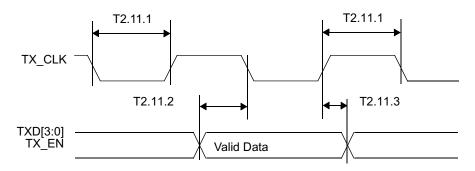
Figure 4-11. 10 Mb/s MII Transmit Timing
