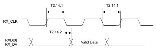
Figure 4-15. 10 Mb/s Serial Mode Receive Timing
