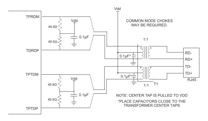
PLACE RESISTORS AND CAPACITORS CLOSE TO THE DEVICE.
