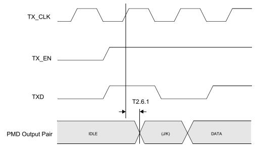
Figure 4-6. 100BASE-TX MII Transmit Packet Latency Timing
