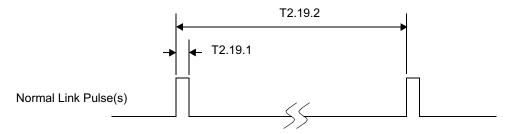
Figure 4-22. 10BASE-T Normal Link Pulse Timing
