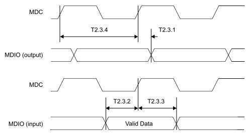
Figure 4-3. MII Serial Management Timing
