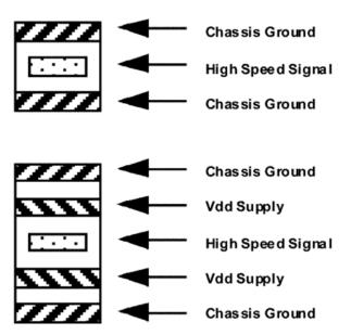
Figure 8-4. Alternative PCB Stripline Layer Stacking
