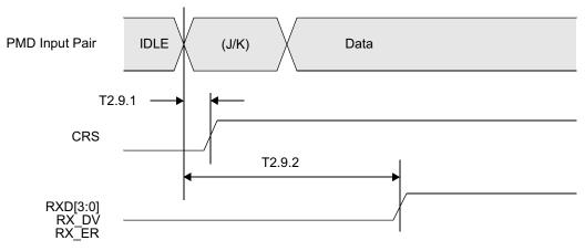
Figure 4-9. 100BASE-TX MII Receive Packet Latency Timing
