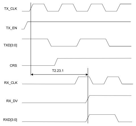
Figure 4-26. 10 Mb/s Internal Loopback Timing
