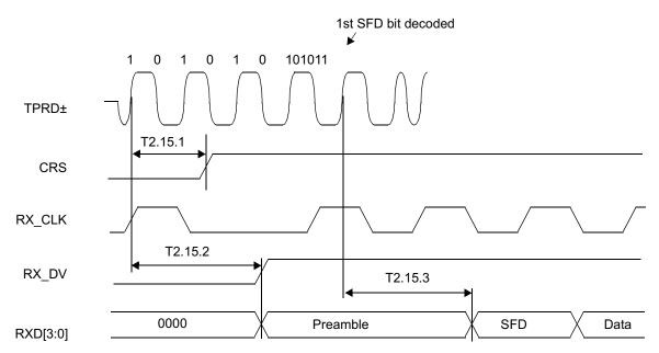
Figure 4-16. 10BASE-T Transmit Timing (Start of Packet)
