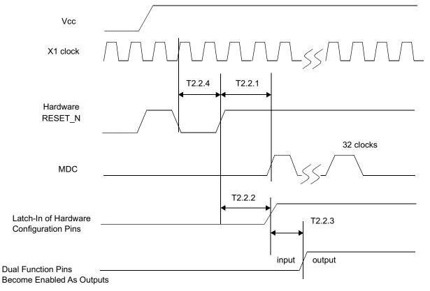
Figure 4-2. Reset Timing
