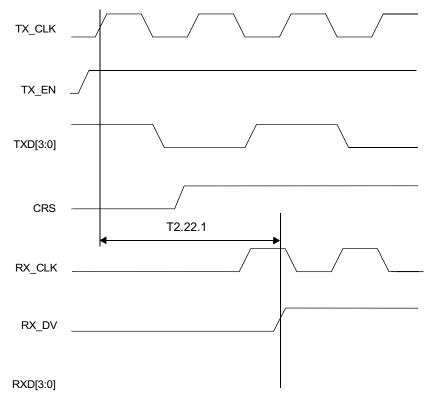
Figure 4-25. 100 Mb/s Internal Loopback Timing
