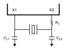
Figure 6-2. Crystal Oscillator Circuit
