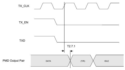
Figure 4-7. 100BASE-TX MII Transmit Packet Deassertion Timing
