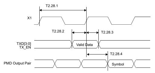
Figure 4-29. Single Clock MII (SCMII) Transmit Timing
