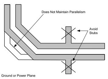
Figure 8-1. Differential Signal Pair - Stubs
