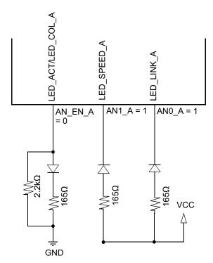
Figure 5-1. AN Strapping and LED Loading Example
