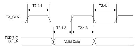
Figure 4-4. 100 Mb/s MII Transmit Timing
