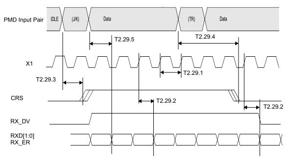
Figure 4-30. Single Clock MII (SCMII) Receive Timing
