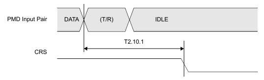
Figure 4-10. 100BASE-TX MII Receive Packet Deassertion Timing
