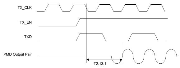
Figure 4-13. 10BASE-T Transmit Timing (Start of Packet)
