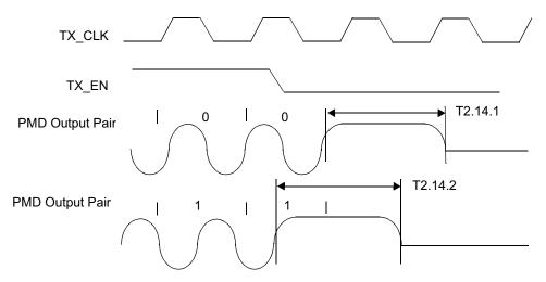
Figure 4-14. 10BASE-T Transmit Timing (End of Packet)
