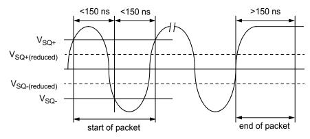
Figure 5-10. 10BASE-T Twisted Pair Smart Squelch Operation
