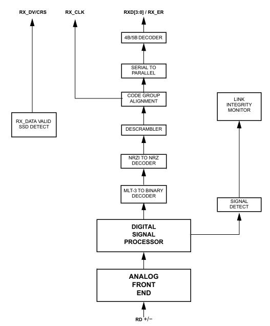
Figure 5-7. 100BASE-TX Receive Block Diagram
