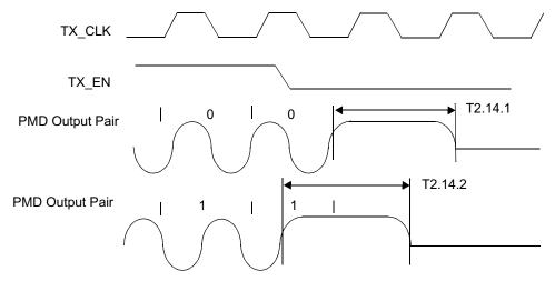
Figure 4-17. 10BASE-T Transmit Timing (End of Packet)
