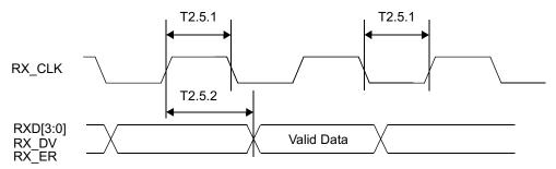
Figure 4-5. 100 Mb/s MII Receive Timing
