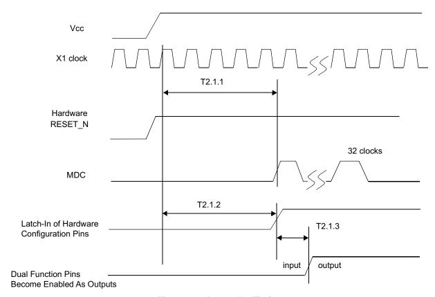
Figure 4-1. Power Up Timing
