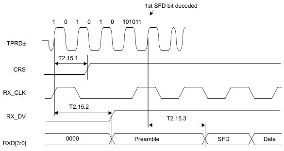
Figure 4-18. 10BASE-T Receive Timing (Start of Packet)
