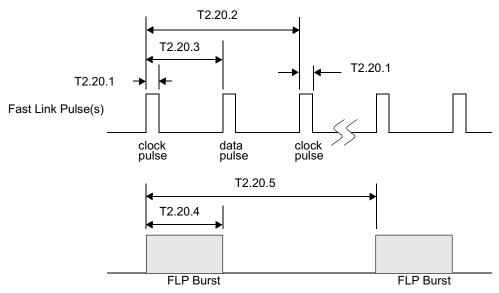
Figure 4-23. Auto-Negotiation Fast Link Pulse (FLP) Timing
