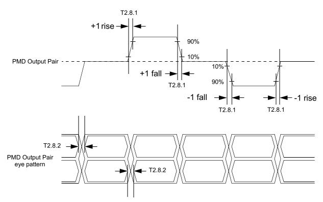
Figure 4-8. 100BASE-TX Transmit Timing (t<sub>R/F</sub> and Jitter)
