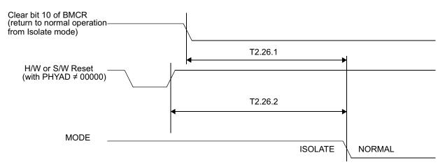
Figure 4-31. Isolation Timing
