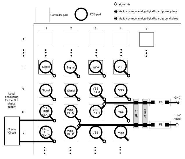
Figure 9-1. PLL Filter Layout
