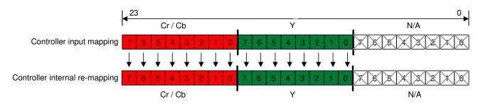
Figure 6-5. 16-Bit YCbCr-880 I/O Mapping
