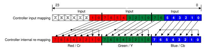
Figure 6-4. RGB-666 and YCbCr-666 I/O Mapping
