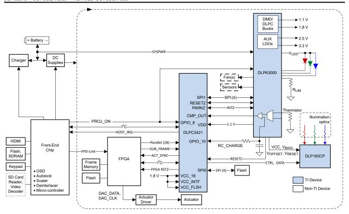
Figure 7-3. Typical Simplified Application Schematic—HD Mode (Using DLPA3000)
