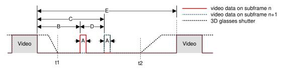
The time offset of DLP Link pulses at the end of a subframe alternates between B and B+D where D is the delta offset.
