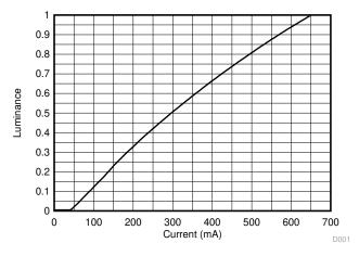
Figure 7-4. Typical Luminance vs Current
