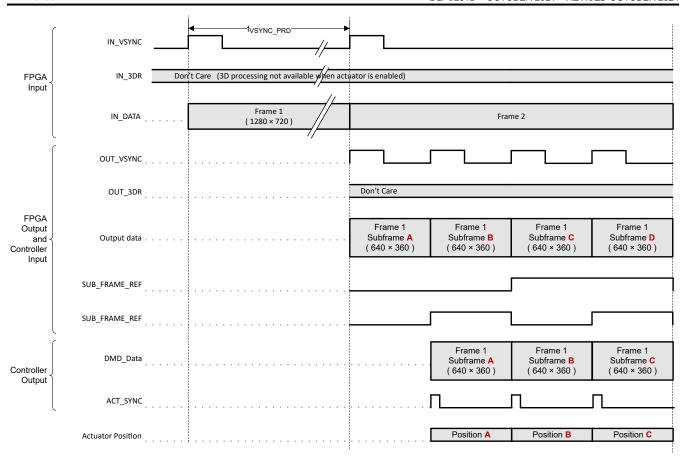
Figure 6-1. HD Actuator Frame and Signal Timing
