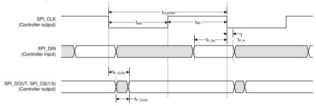
Figure 5-9. Flash Interface Timing
