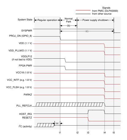
Figure 8-4. Normal Park Power-Down Waveforms for HD Mode
