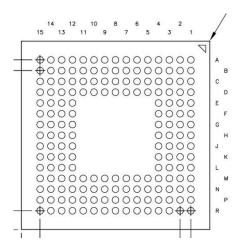
Figure 4-1. ZVB Package 176-Pin NFBGA Bottom View
