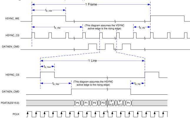
Figure 5-7. Parallel Interface Video Frame Timing
