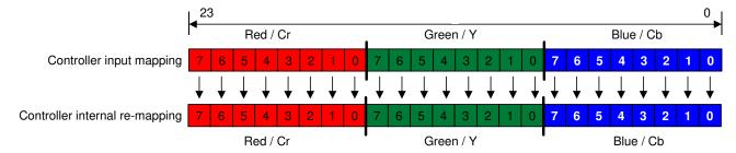
Figure 6-3. RGB-888 and YCbCr-888 I/O Mapping
