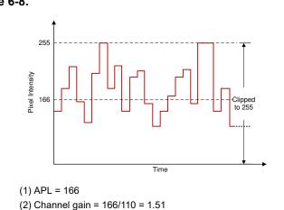
Figure 6-8. Source Pixels for a Color Channel
