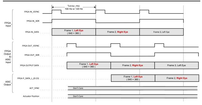
Figure 6-2. 3D Frame and Signal Timing
