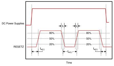
Figure 5-6. Power-Up and Power-Down RESETZ Timing
