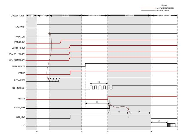
Figure 8-2. System Power-Up Waveforms for HD Mode
