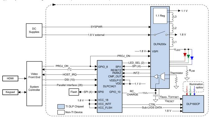
Figure 7-1. Typical Simplified Application Schematic—nHD Mode (Using DLPA200x)
