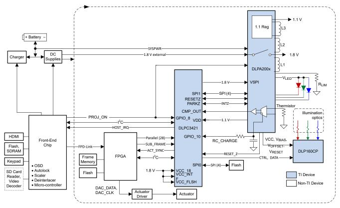
Figure 7-2. Typical Simplified Application Schematic—HD Mode (Using DLPA200x)
