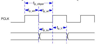
Figure 5-8. Parallel Interface Pixel Timing
