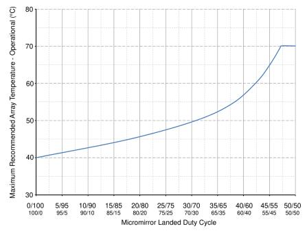
Figure 5-1. Maximum Recommended Array Temperature—Derating Curve
