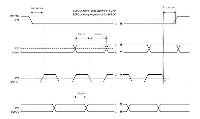
Figure 5-3. SCP Timing Parameters
