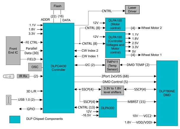
Figure 7-2. Typical Full HD Laser Phosphor Application
