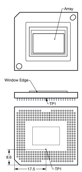
Figure 6-1. DMD Thermal Test Point
