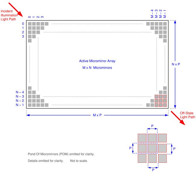
Figure 5-10. Micromirror Array Physical Characteristics
