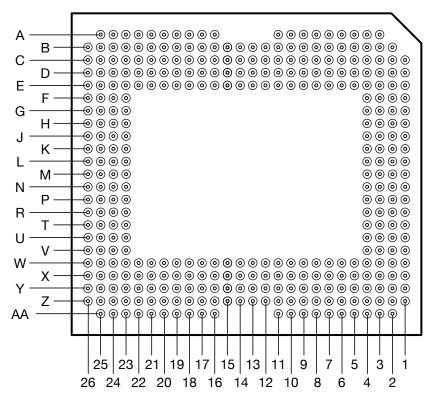
Figure 4-1. FYU Package (350-Pin) Bottom View
