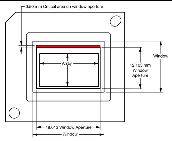
Figure 5-2. Illumination Overfill Diagram—Critical Area
