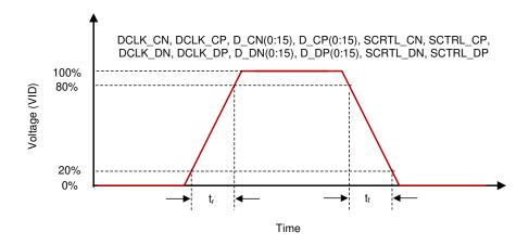
Figure 5-6. LVDS Rise and Fall Times
