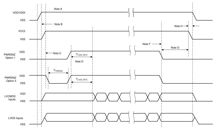
Figure 8-1. DMD Power Supply Sequencing Requirements
