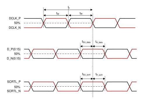
Figure 5-7. LVDS Timing Parameters
