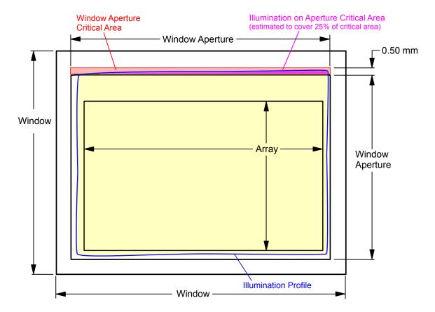
Figure 6-2. Window Aperture Overfill Example
