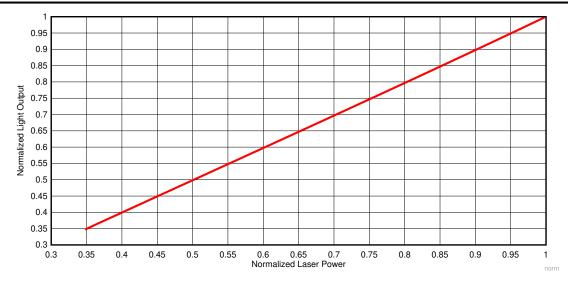
Figure 7-3. Normalized Light Output vs. Normalized Laser Power for Laser Phosphor Illumination
