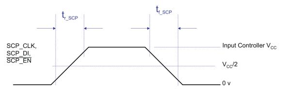
Figure 5-6. Serial Communications Bus Waveform Requirements
