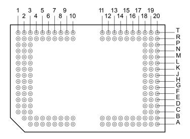
Figure 4-1. FYA Package 149-Pin Bottom View
