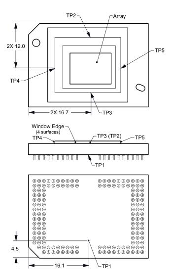
Figure 6-1. Thermal Test Point Location
