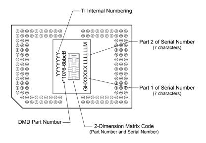
Figure 9-2. DMD Marking (Device Top View)
