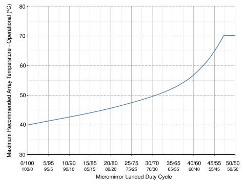
Figure 5-1. Maximum Recommended DMD Temperature—Derating Curve
