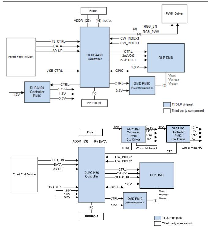
Figure 7-1. Typical DLPC4430 Application (LED Top, LPCW Bottom)
