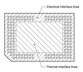
Figure 5-10. System Interface Loads
