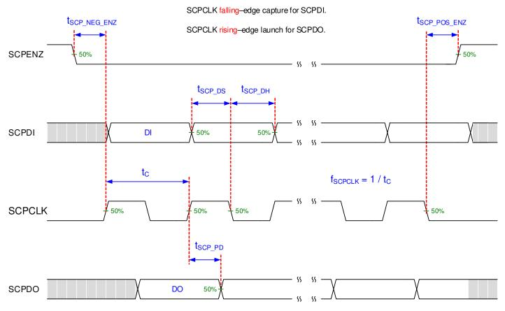
Figure 5-2. SCP Timing Parameters
