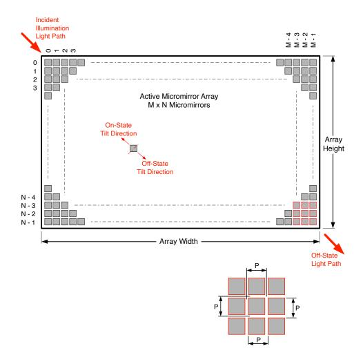
Figure 5-15. Micromirror Array Physical Characteristics
