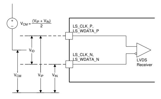
Figure 5-7. LSIF Voltage Requirements
