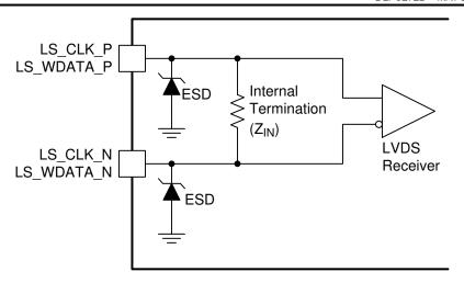
Figure 5-8. LSIF Equivalent Input
