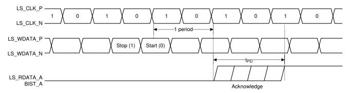
Figure 5-3. Switching Characteristics
