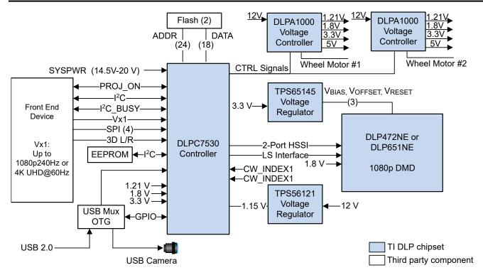
Figure 7-1. Typical Full HD Laser Phosphor Application Diagram
