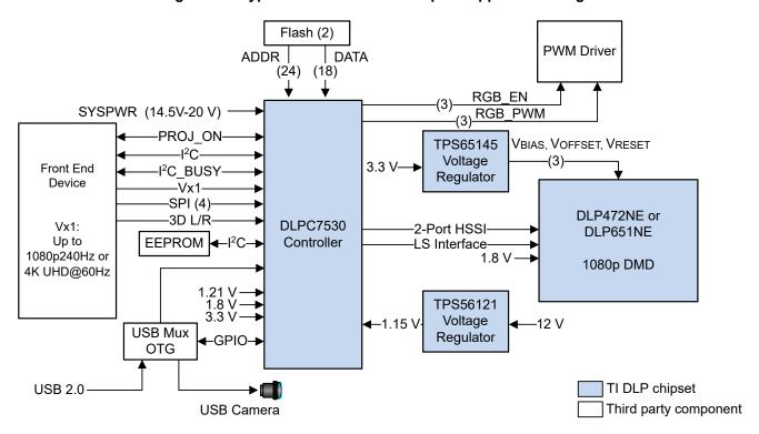
Figure 7-2. Typical Full HD LED Application Diagram
