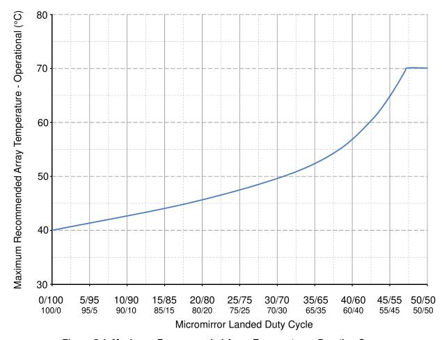
Figure 5-1. Maximum Recommended Array Temperature—Derating Curve
