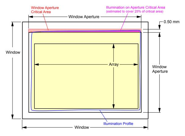
Figure 6-2. Window Aperture Overfill Example
