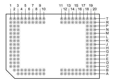
Figure 4-1. FYW Package 149-Pin PGA Bottom View
