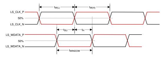
Figure 5-5. LSIF Timing Requirements
