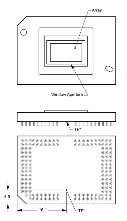
Figure 6-1. DMD Thermal Test Points
