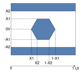
Figure 5-12. HSSI Eye Characteristics
