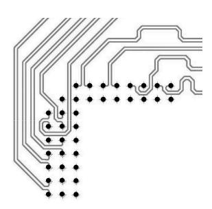
Figure 9-1. Example HSSI PCB Routing
