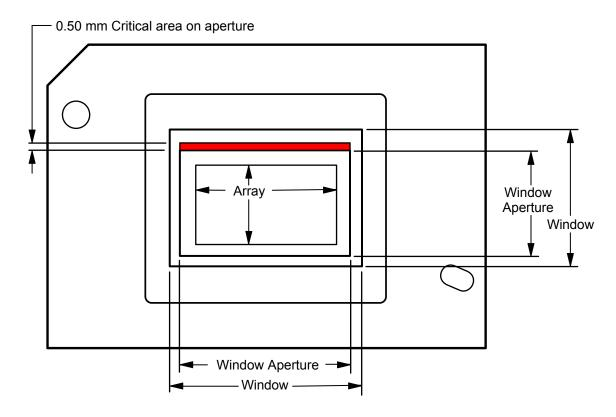
Figure 5-2. Illumination Overfill Diagram—Critical Area
