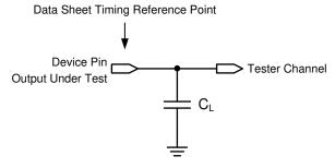
Figure 6-5. Test Load Circuit for Output Propagation Measurement
