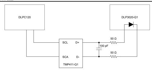
Figure 7-1. Temperature Sense Diode Typical Circuit Configuration
