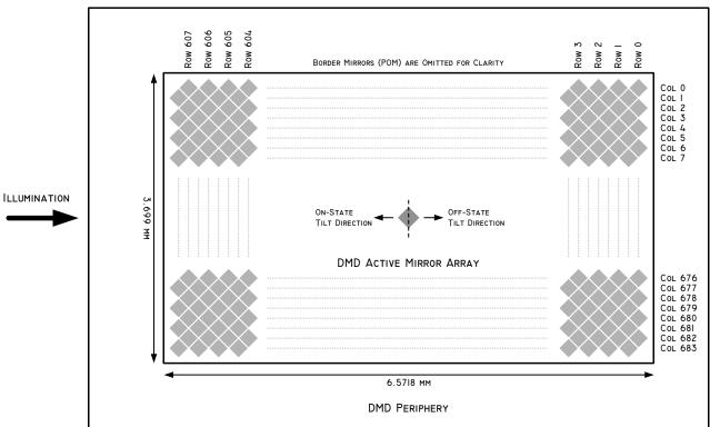
Figure 6-7. Micromirror Array Physical Characteristics
