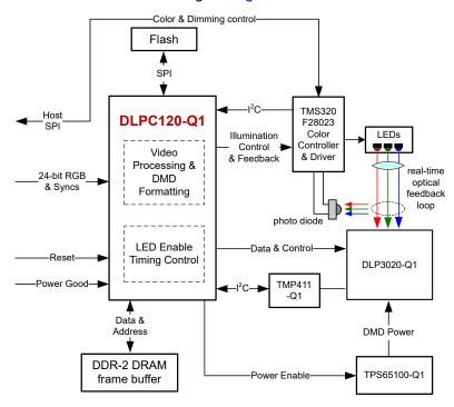
Figure 8-1. HUD Reference Design Block Diagram
