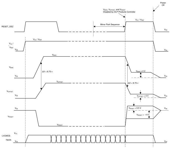
Note 1:  $\pm 8.75$ -V delta,  $\Delta V$ , shall be considered the max operating delta between  $V_{BIAS}$  and  $V_{OFFSET}$ . Customers may find that the most reliable way to ensure this is to power  $V_{OFFSET}$  prior to  $V_{BIAS}$  during power up and to remove  $V_{BIAS}$  prior to  $V_{OFFSET}$  during power down.
