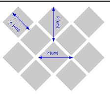
Figure 6-8. Mirror (Pixel) Pitch
