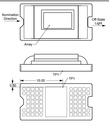
Figure 7-8. Thermocouple Location
