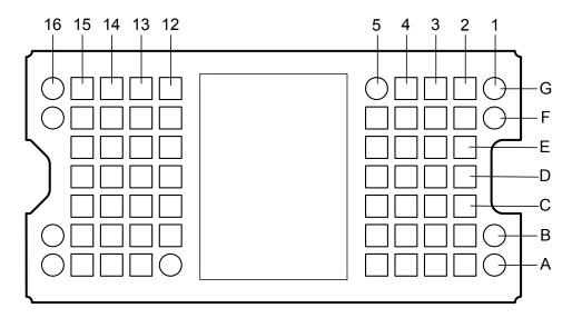
Figure 5-1. FQR Package, 64-Pin LGA (Bottom View)
