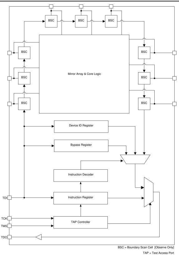
Figure 7-7. JTAG Functional Block Diagram
