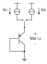
Figure 7-2. Temperature Measurement Theory
