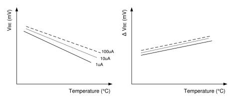
Figure 7-3. Example of Delta VBE vs Temperature
