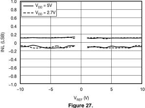
INTEGRAL NONLINEARITY vs  $V_{REF}$  BIPOLAR MODE
