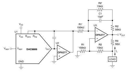
Figure 43. Programmable Bidirectional Current Source Circuit
