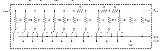
Figure 38. Equivalent R-2R DAC Circuit
