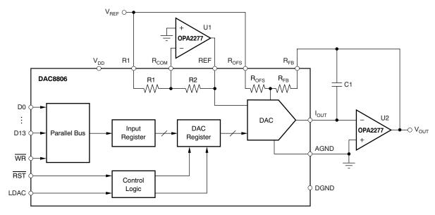
Figure 42. Bipolar Output Circuit
