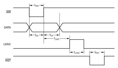
Figure 40. DAC8806 Timing Diagram
