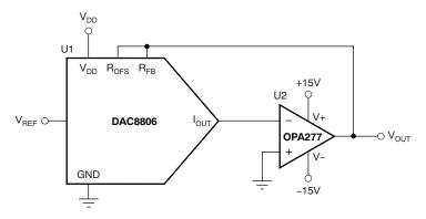
Figure 39. Voltage Output Configuration
