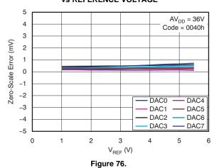
**ZERO-SCALE ERROR vs REFERENCE VOLTAGE**
