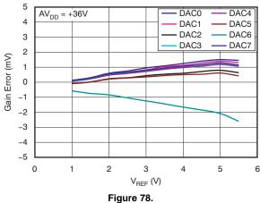
**GAIN ERROR vs REFERENCE VOLTAGE**
