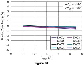
BIPOLAR ZERO ERROR VS REFERENCE VOLTAGE
