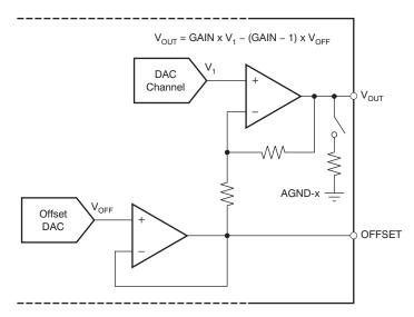
Figure 96. Output Amplifier and Offset DAC
