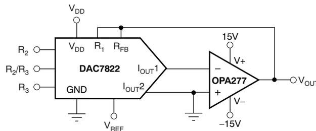
**Figure 38. Voltage Output Configuration**
