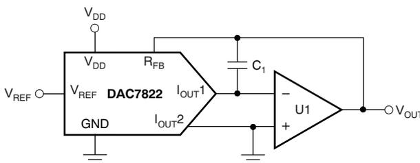
**Figure 39. Gain Peaking Prevention Circuit with Compensation Capacitor**
