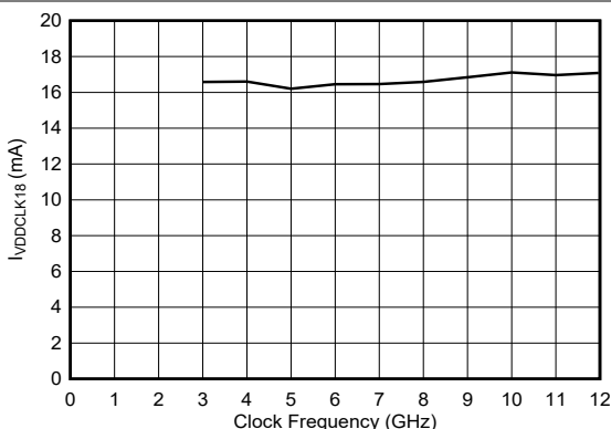
Figure 6-209. VDDCLK18 Current vs Clock Frequency
